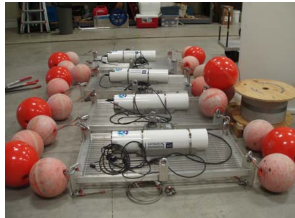
Figure 7. This figure shows the 4 SWIPS units with external battery packs mounted on sleds prior to deployment -Courtesy of Nathan Hawley, GLERL
