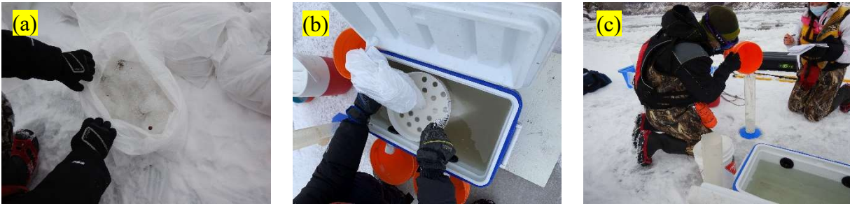
Figure 4. Images showing the anchor ice volume measurement methodology, (a) anchor ice transferred into a plastic bag, (b) bagged sample submerged into cooler full of water using a pressing tool and, (c) measuring the volume of the overflow using a graduated cylinder
