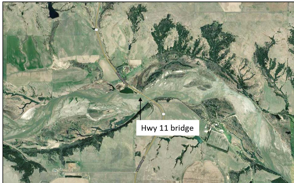
Figure 6. The Niobrara River at a reach including the Highway 11 Bridge, 8.5 km upstream of Spencer Dam. The river width here is about 153 m (Source: adapted from Google Earth)
