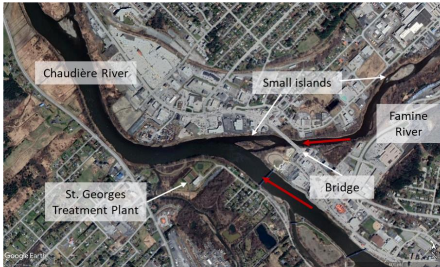
Figure 9. FA confluence showing small islands as well as the bridge present in the tributary and the water treatment plant adding its water to the CH River. Red arrows are showing the direction of the flow.
