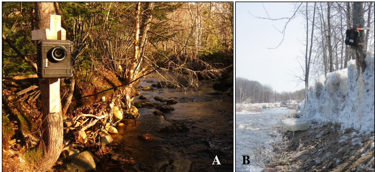
Figure 2. (A) Canon 20D camera installed on a tree on the side of a small stream in the fall and (B) Camera almost damaged by a major spring breakup event on the side of a large stream.
