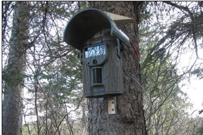
Figure 8. Camera installation including screwed-in mount, snow protection “hat”, and security cable with lock.
