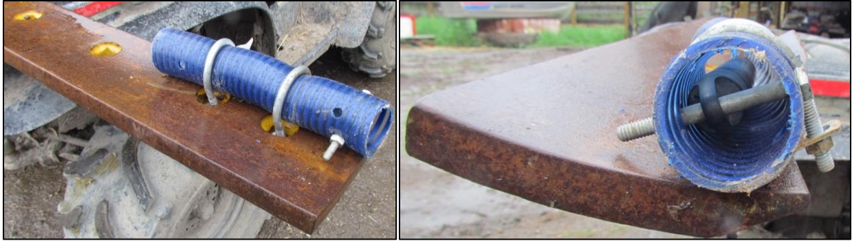
Figure 5. Anchoring system for autonomous water level and temperature loggers (PVC tube tied to a grader blade using U-bolts)
