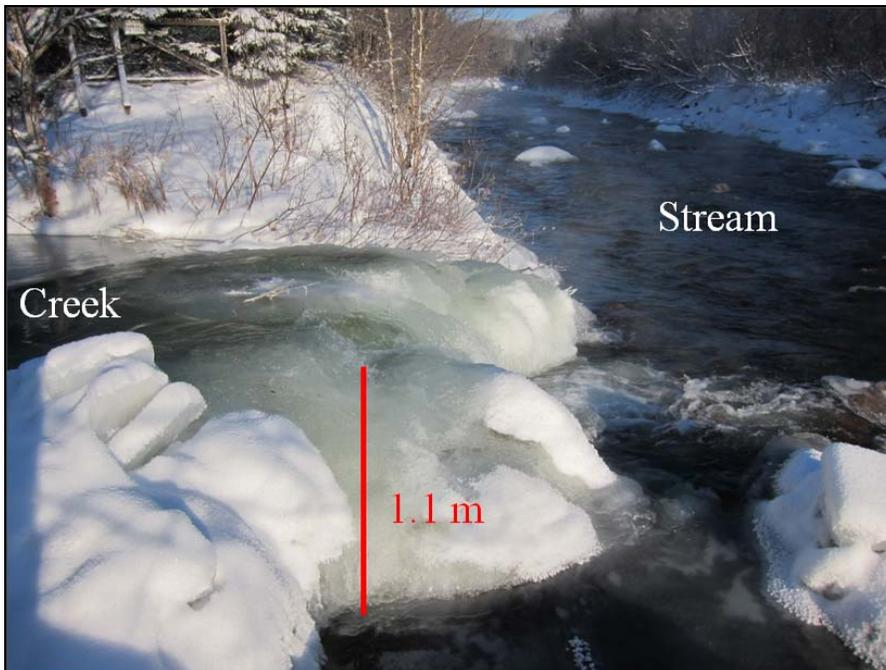
Figure 6. ID at the exit of the Creek (Stream flowing toward the camera) on December 16, 2010.
