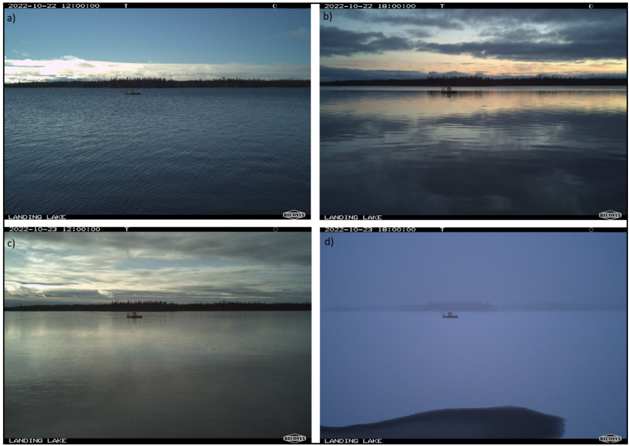
Figure 5. The freeze-up of Landing Lake- south facing from the northern shore of the lake. The images show a) open-water, b) border ice, progressing from the southern, shallower portions of the lake, c) a solid, stable cover of skim ice, and d) the onset of slush formation along the shoreline due to increasing snow loads on the lake surface.
