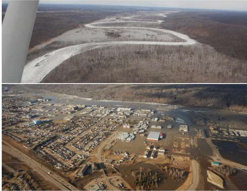
Figure 8. Top: looking downstream on the Clearwater River at Draper and towards downtown Fort McMurray on April 27, 2020, backwater from the ice jam has filled the Clearwater River from valley wall to valley wall. Bottom: flooding in downtown Fort McMurray on April 28, 2020.
