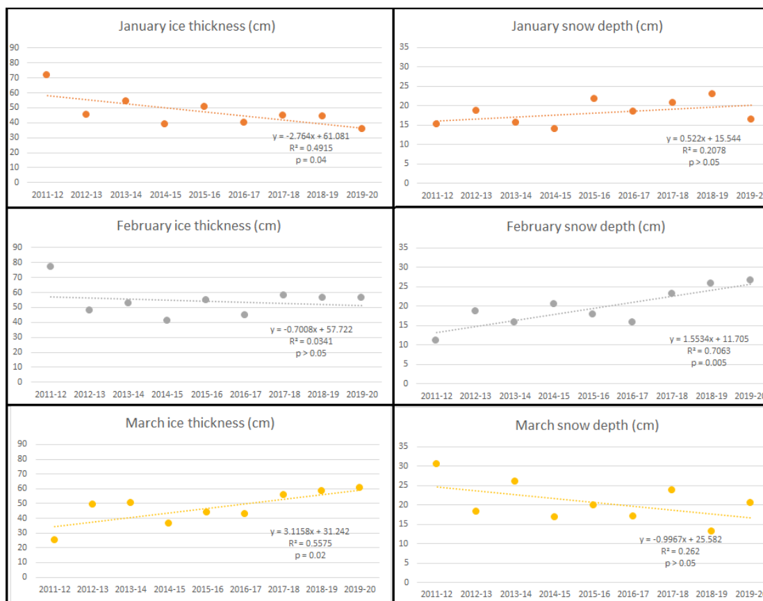
Figure 4. Linear regression of average monthly ice thickness (left hand column) and snow depth (right hand column) for entire region for each ice season.
