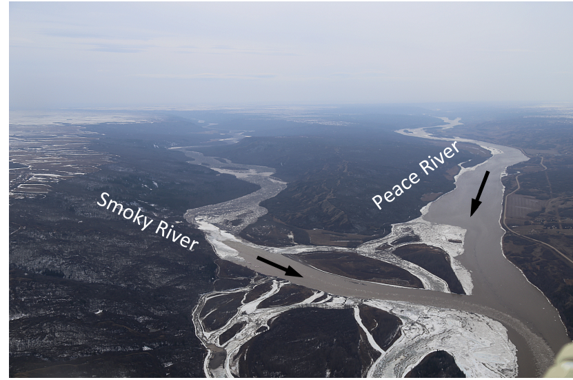
Figure 7. Toe of an 18 km ice jam on the Smoky River (left) on Apr 24, 2018 15:25 MDT, 2 km from the confluence with the Peace River (right) which had broken up thermally on Apr 12.
