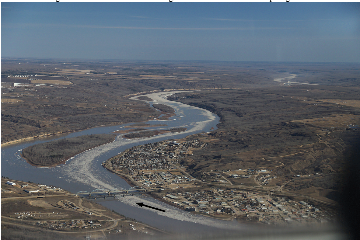
Figure 10. Looking downstream from the Town of Peace River at an ice run on Apr 26, 2018 10:57 MDT that originated from the Smoky River and produced the peak flow in spring 2018.
