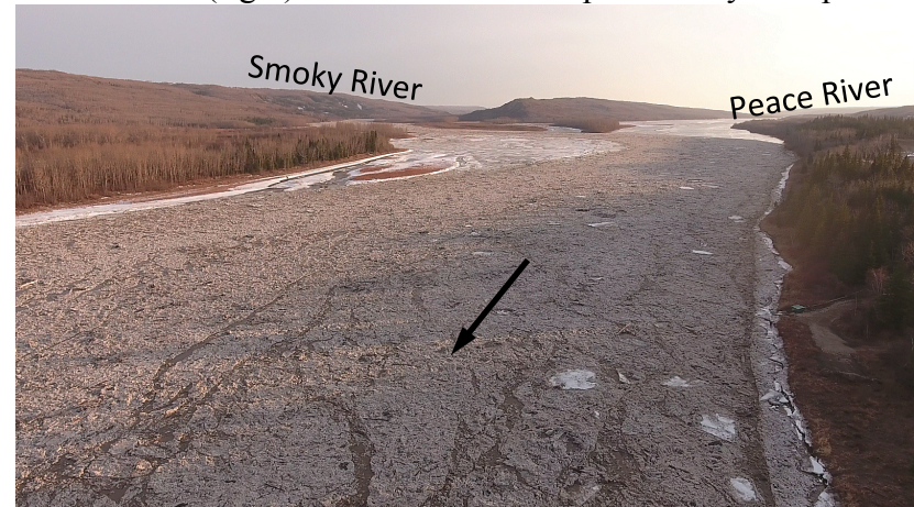
Figure 8. Smoky River 18 km long ice jam releasing into the Peace River on Apr 24, 2018 21:17 MDT (about 2.25 hours after the start of the release).
