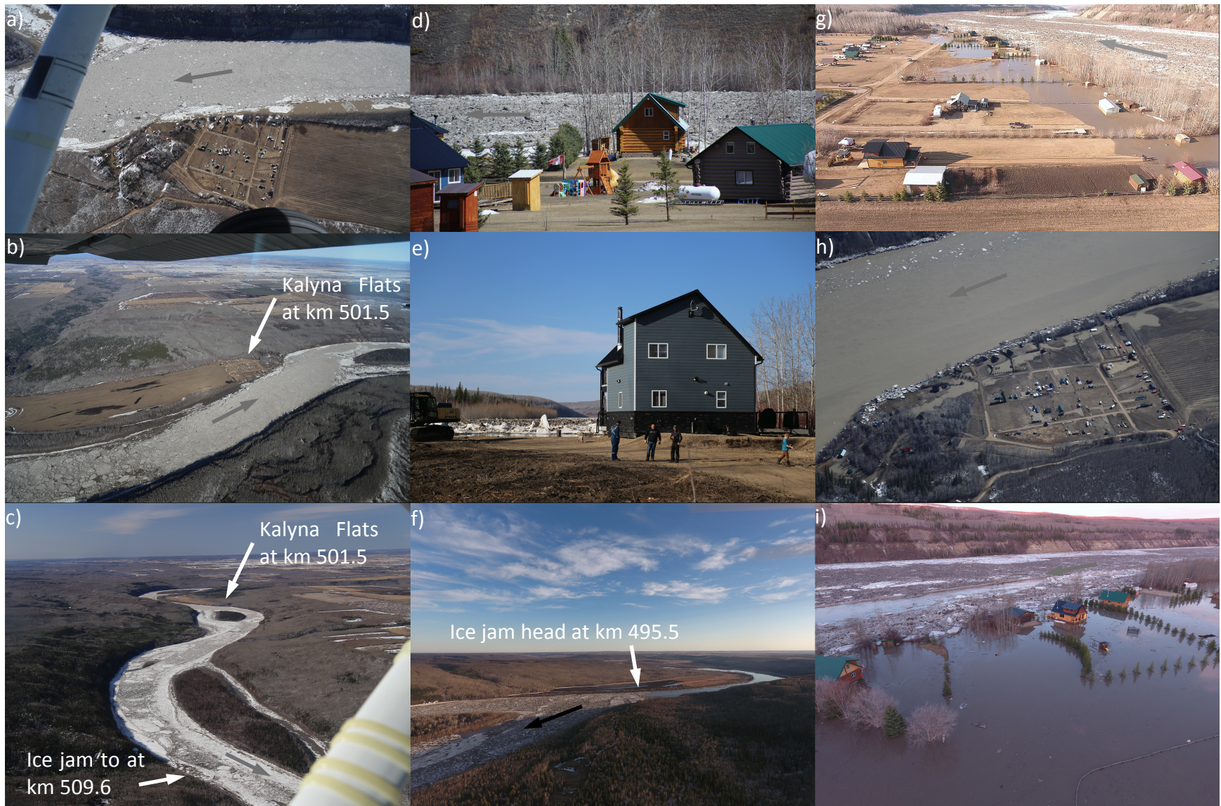
Figure 12 a,b) Ice jam formation c) toe at km 509 on Apr 25, 2018 09:47 MDT. d,e) increasing water levels at Kalyna Flats. f) Head of ice jam at km 495.5 on Apr 25, 2018 20:09 MDT. g,h,i) flooding at Kalyna Flats.
