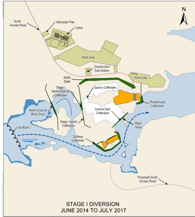
Figure 1. Keeyask Project Stage 1 River Diversion Strategy
