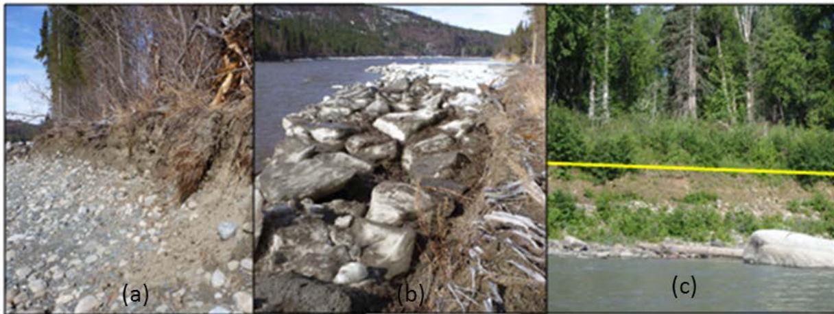
Figure 7. Illustrations of ice-block shearing of river banks: (a) and (b) photos taken on May 5, 2012 of ice-block shearing of a mid-channel island at Mile 185.9; and, (c) a photo taken of sheared bank vegetation, on July 24, 2013 at Mile 109.
