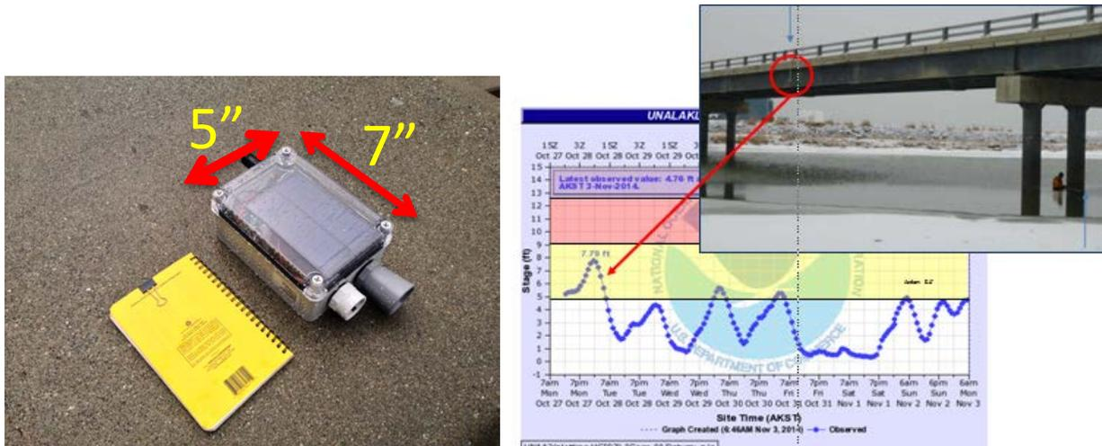
Figure 6. Photograph of a the APRFC low cost telemetered stage gage (left) with a photograph of a typical installation on a tidally affected bridge.
