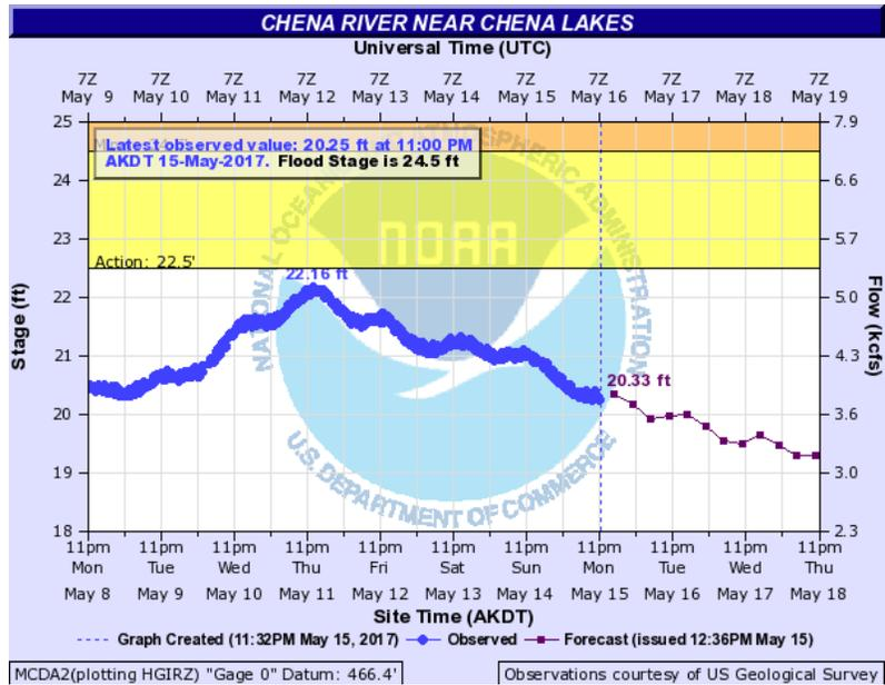
Figure 2. Example APRFC open water season hydrograph. The primary plotted variable is river stage on the left axis with discharge included on the right axis. Flood stages are highlighted in the plot to provide users with information related to flood impacts.
