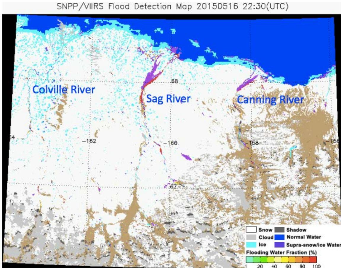
Figure 4. Example SNPP/VIIRS JPSS River Ice and Flood Product from May 16<sup>th</sup> 2015. This image shows an area of widespread flooding and water over snow and ice along the Sagavanirktok River on the North Slope of Alaska.
