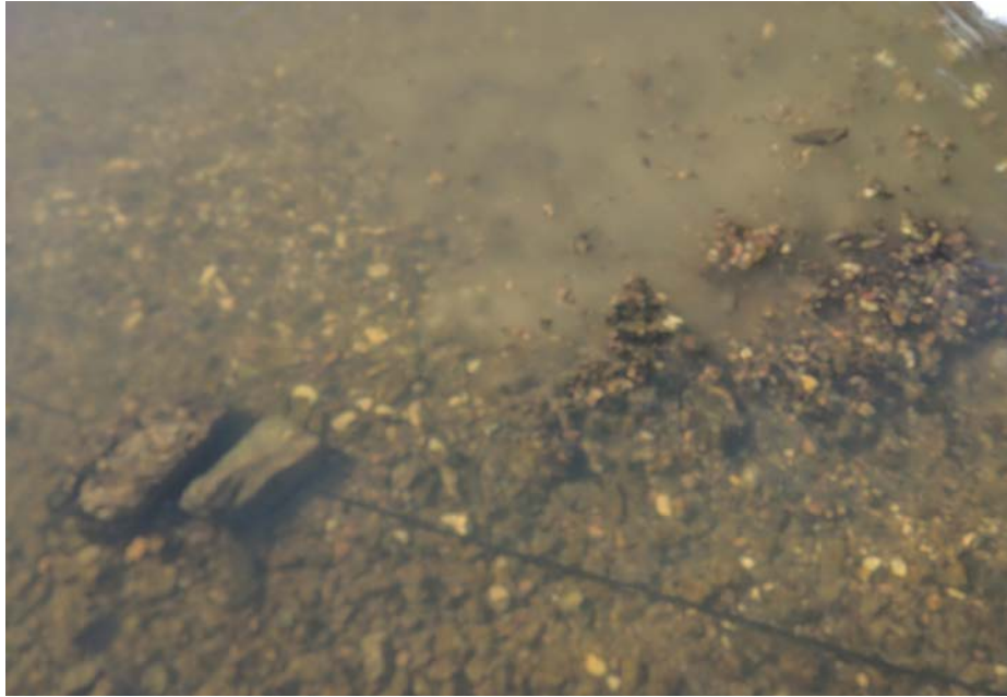
Figure 5. Image of DTS cable going under an anchor-ice mass.
