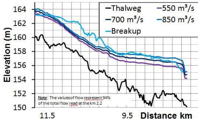
Figure 3. Water level estimated by LiDAR (light blue) at breakup compared to simulated values under open water conditions.
