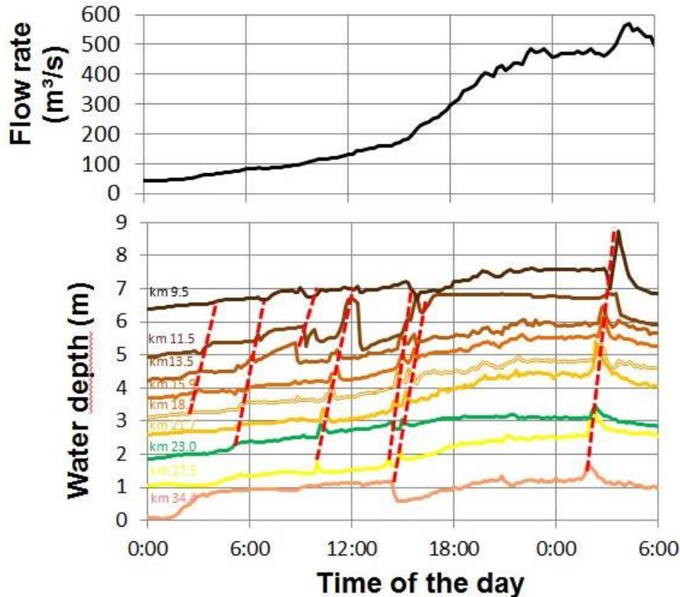
Figure 2. Flow rate, water levels (various colours) and javes (red lines) measured at breakup from April 15<sup>th</sup> to April 16<sup>th</sup>, 2014
