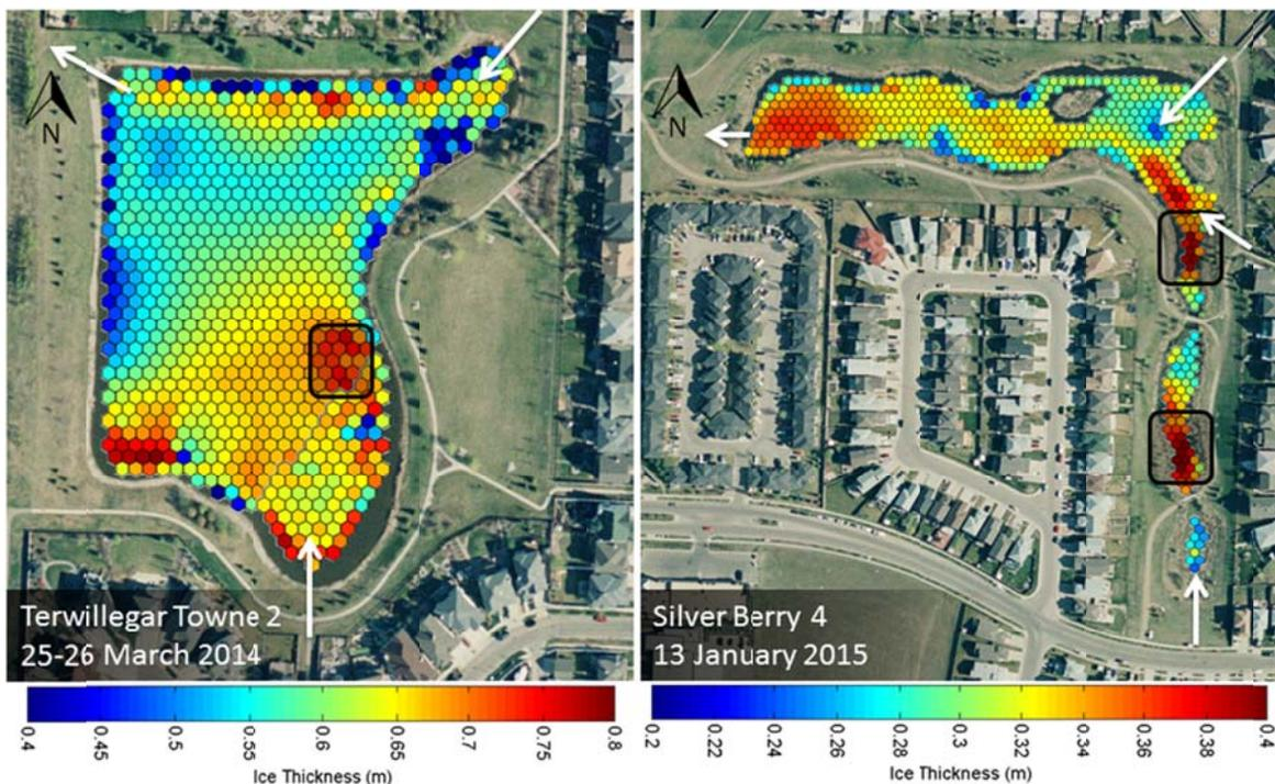
Figure 1. Processed GPR ice thickness surveys showing thinner ice at inlets and thicker ice near the outlets and rinks (inlets and outlets indicated by white arrows and rinks by black rectangles).
