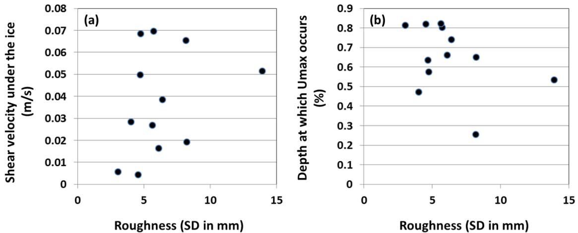
**Figure 3.** Relation between (a) the shear velocity and (b) the depth at which the maximum velocity occurs against the standard deviation of ice cover roughness.
