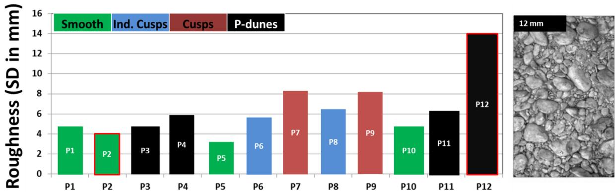
**Figure 2.** DEM standard deviation for the 12 under ice cover surfaces. For comparison, a gravel bed surface with a standard deviation of 12 is also shown.
