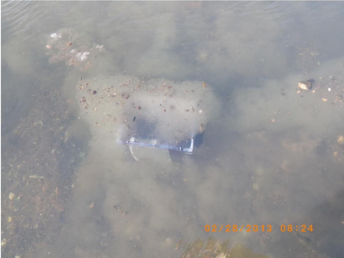
Figure 6. Ice blockage of experimental wedge wire screen elements mounted in an acrylic box on the morning of 2/28/13. It was impossible to distinguish between ice formed on the wedge wire screen and anchor ice formed on the surrounding bottom.
