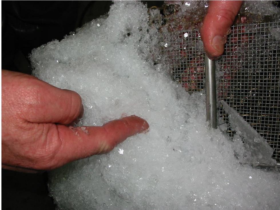
Figure 3. Frazil freshly accumulated onto a screen (background) during an intake blockage tank experiment (from Chen et al 2004). 15 minutes into experiment
