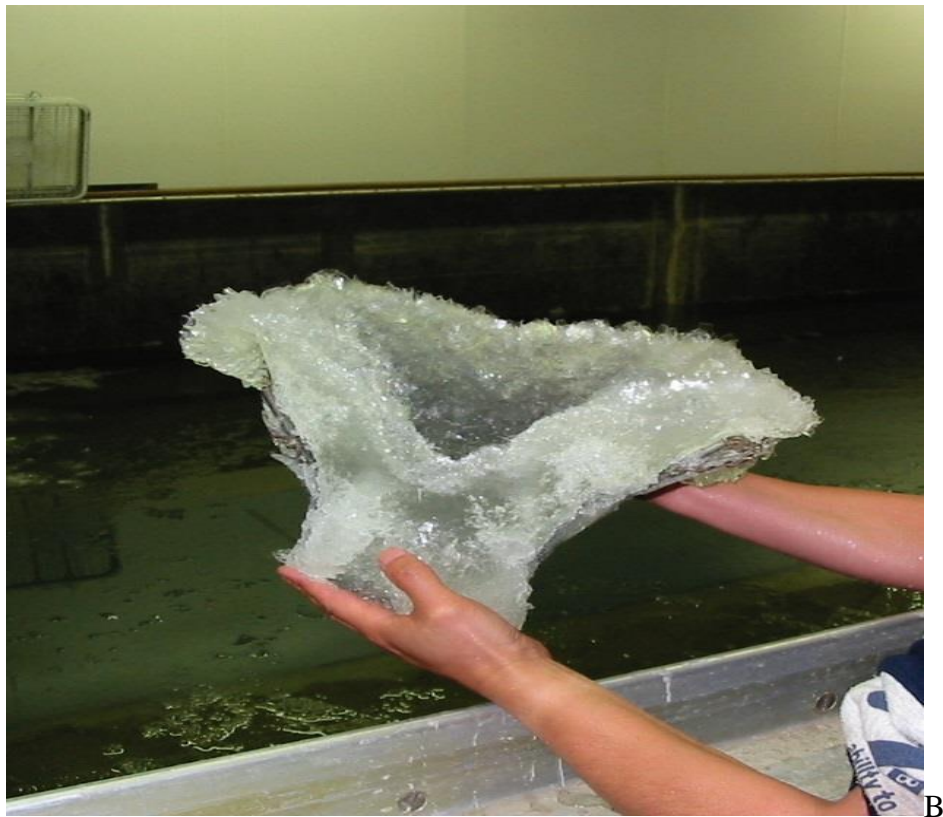
Figure 5. (A) Early stage of complete frazil ice blockage of cone-shaped intake from tank experiments of Chen et al. (2004). (B) Collapsed ice mass from same cone after about 60 minutes of model intake operation. Crystals on the rim of the ice mass show evidence of in situ growth. Porosity varied through this ice mass (from Chen et al. 2004)
