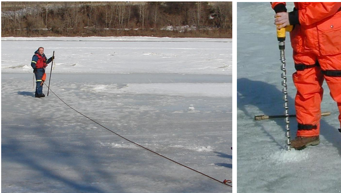
Figure 3. Team member secured and checking ice integrity (left), checking ice thickness directly using a 5 cm drill bit (right).
