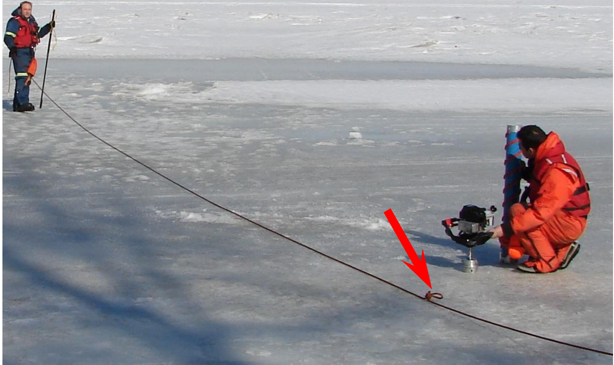
Figure 5. Figure 8 knot (on a bight) in tether rope approximately 1/3 to 1/2 of the way from the free end.
