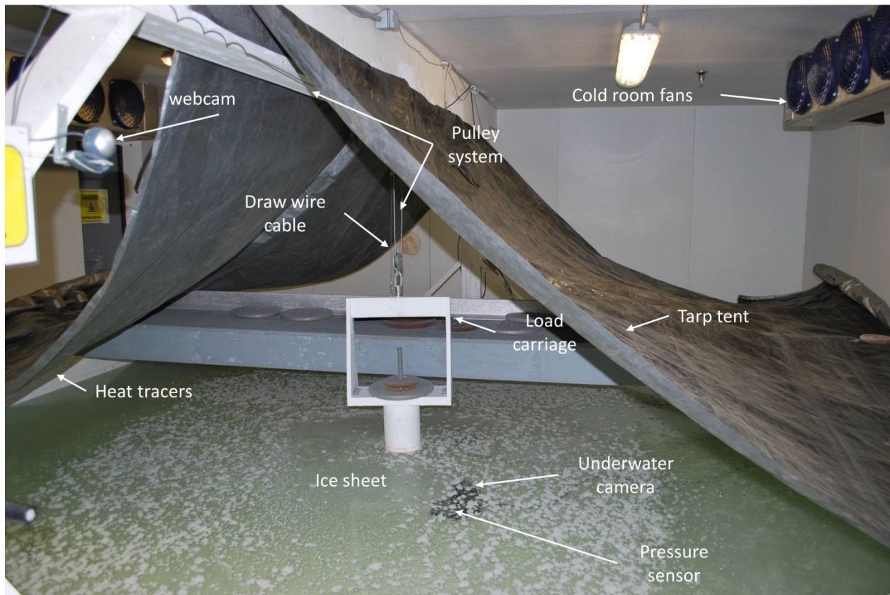
Figure 1. Photograph showing the setup and the location of the instrumentation used for the ice creep experiments.
