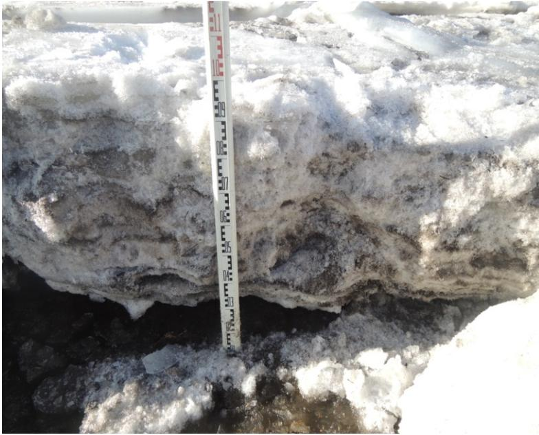
Figure 3: Example of frazil slush accumulation.
