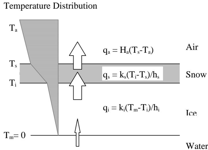
**Figure 4.1** Heat Flux Through an Ice Cover
