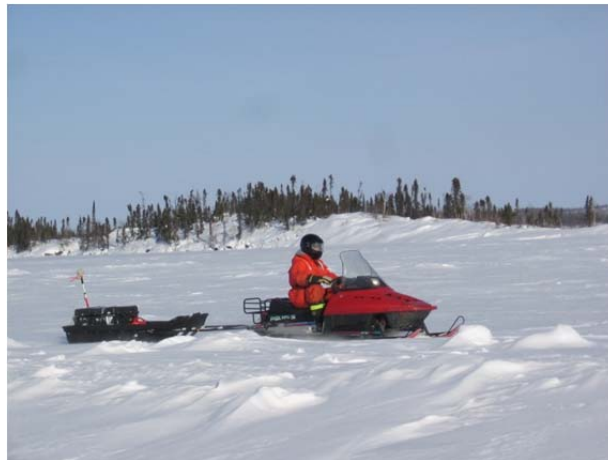
Figure 2. Snowmobile with SIR 8 GPR and 120 MHz antenna
