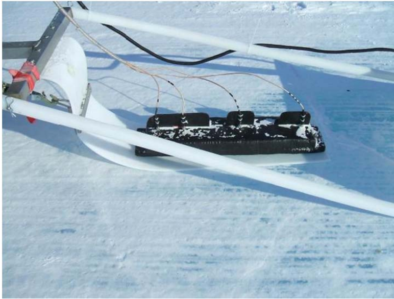
Figure 8. Ice Road Radar multi-channel ice antenna
