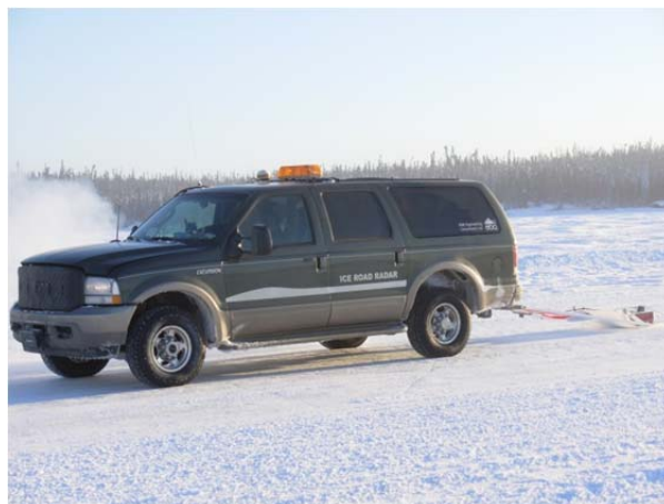
Figure 1. Ice Road Radar Truck with SIR 8 GPR and 500 MHz antenna
