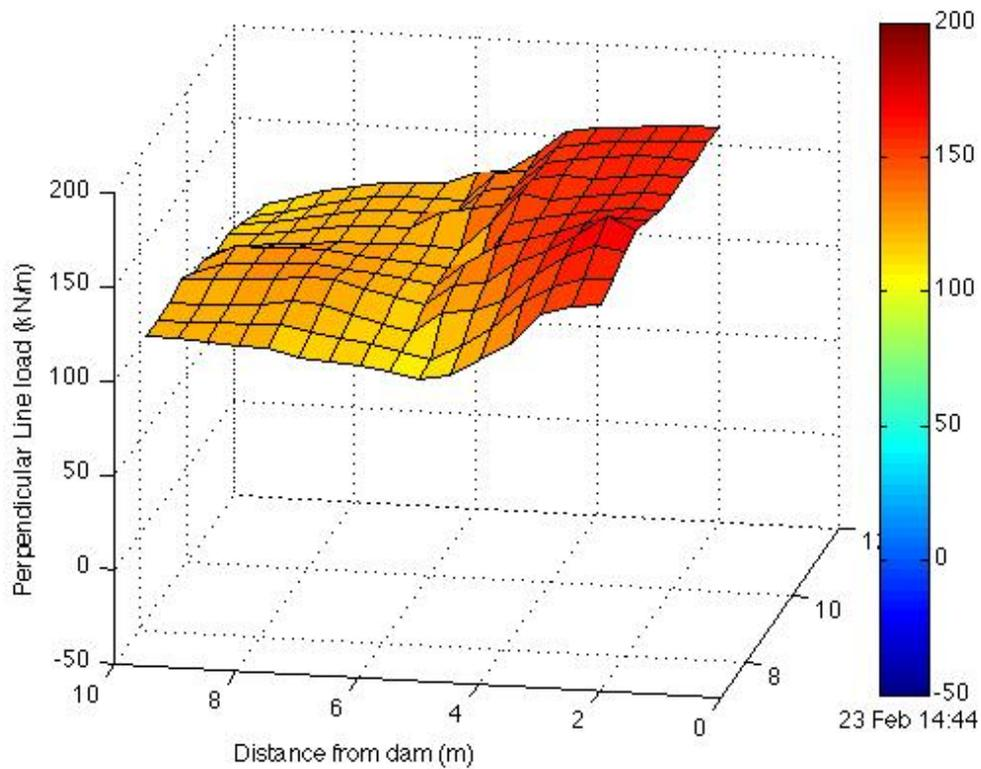
Figure 10. Spatial variation of line load at time of maximum thrust.
