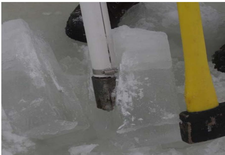
Figure 2. Biaxial gauge no 18 held in place by 2" white PVC pipe being removed from ice on Feb. 6<sup>th</sup>.
