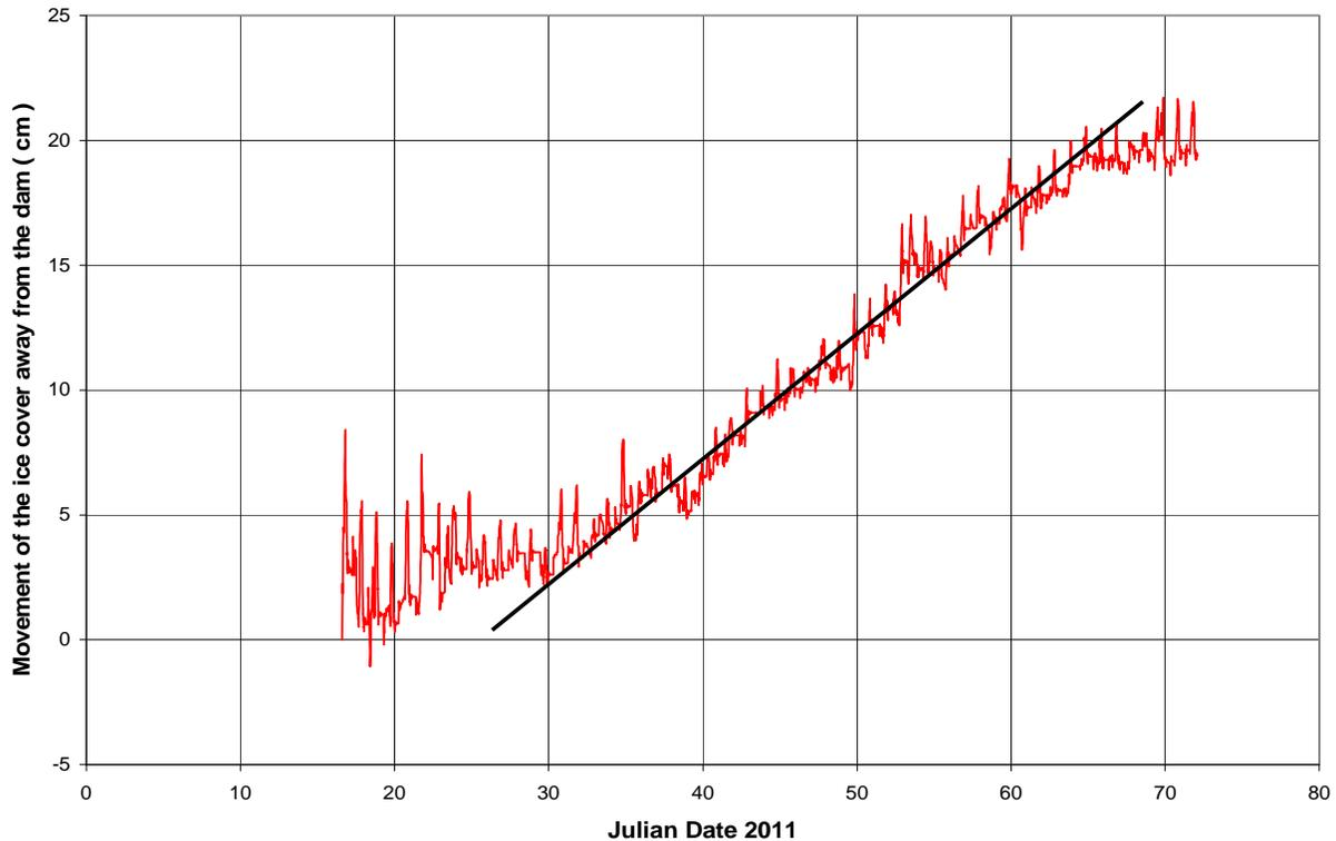
Figure 6. The offshore movement of the main ice sheet as a result of ice formation in the ballycatter fissure. Each peak marks a change in forebay elevation within the reservoir.
