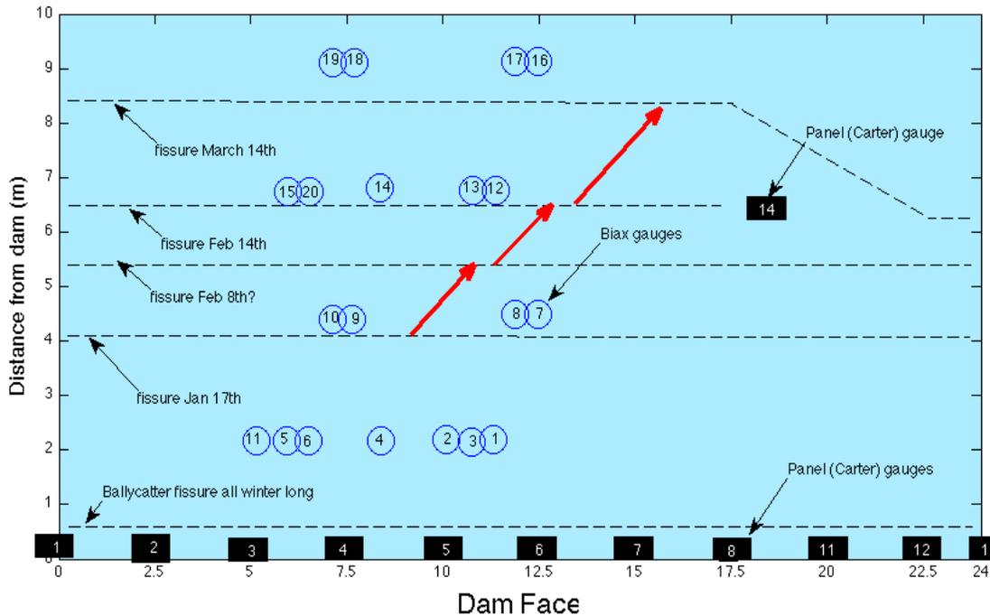
Figure 4. Location of fissures in Barrett ice sheet as well as location of biaxial gauges (circles) and Carter panels (rectangles).
