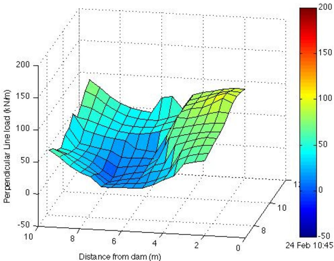
Figure 9. Spatial variation of line load during a transition period. (X-axis is distance along the dam)
