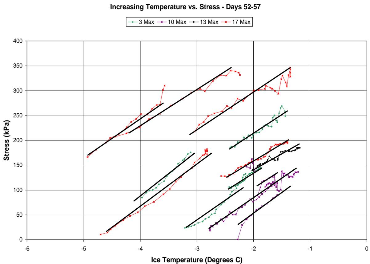
Figure 8. Increase in principal stress measured by biaxial gauges as a function of increase in ice temperature. Observed deviations from the best fit lines are primarily due to short lived fluctuations in forebay elevation.
