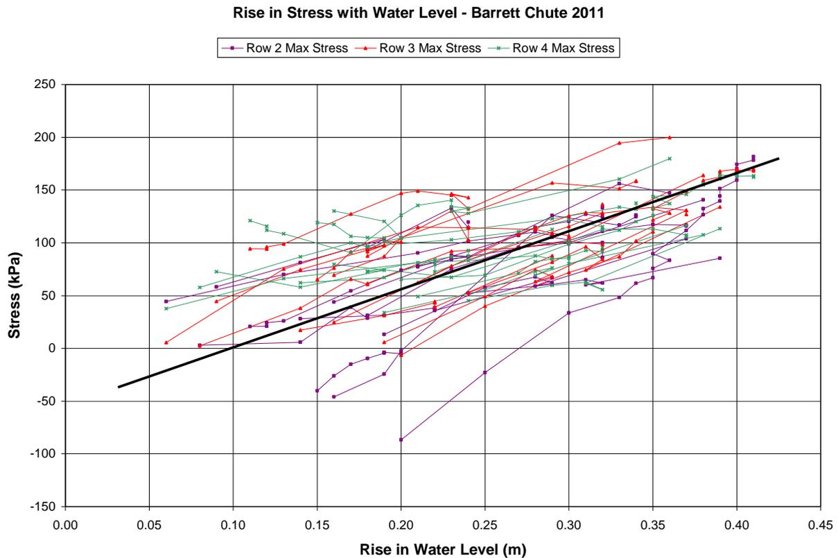
Figure 5. Increase in principal stress as a function of the rise of forebay elevation.
