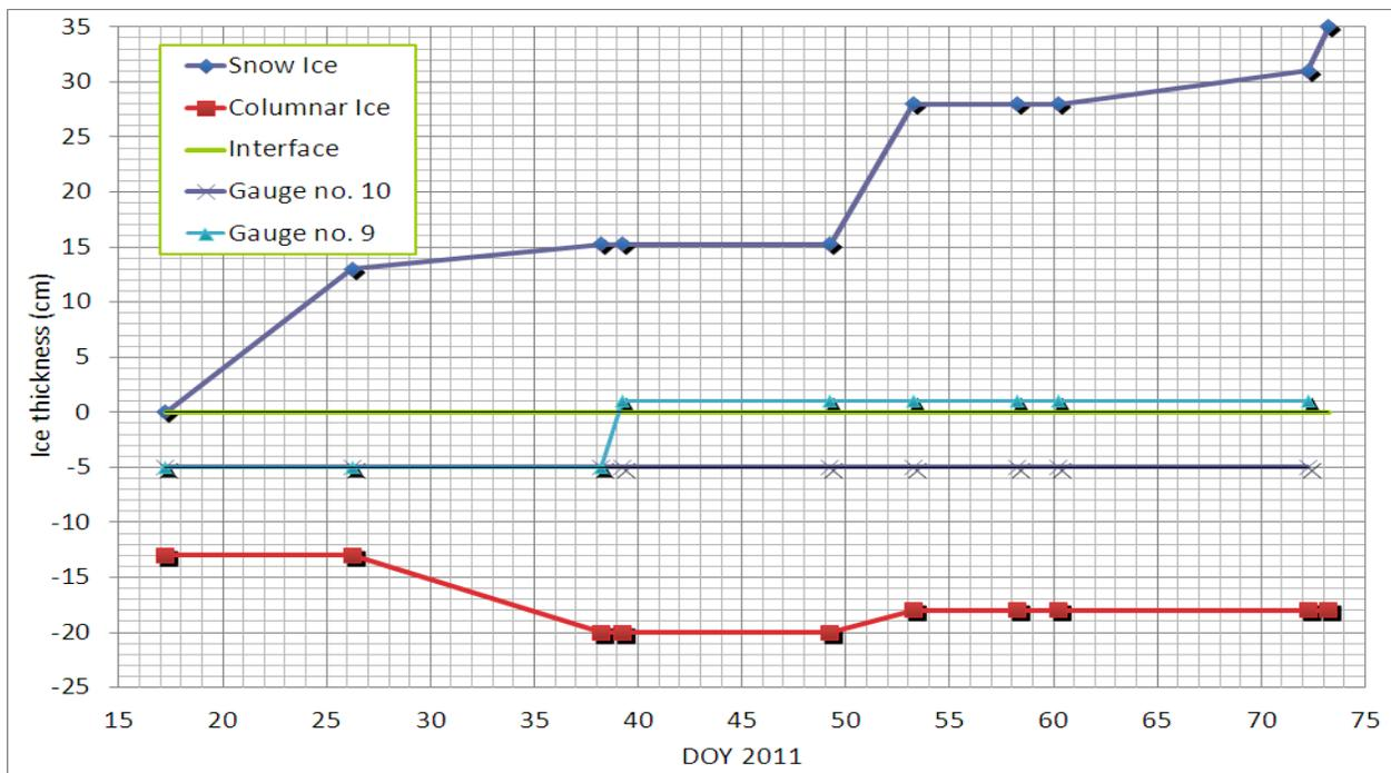
Figure 3. Ice growth separated by an interface at row no. 2 located 4.6 m from the dam face indicating biaxial gauge placement (Table 1). (DOY = Day of Year = Julian day).
