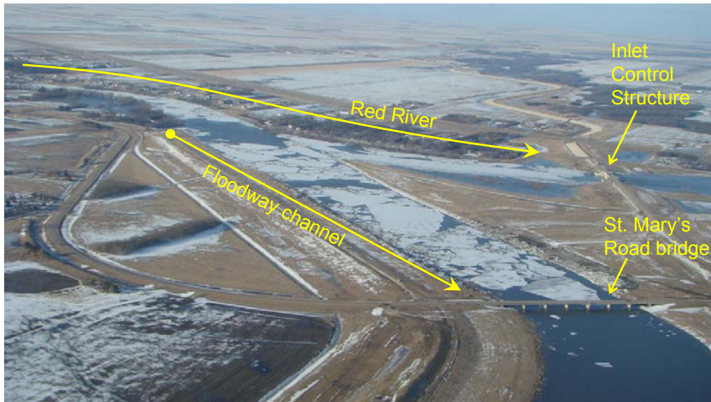
Figure 7. River ice entering the Floodway channel during a necessary operation of the Floodway during the onset of spring flooding in 2009.
