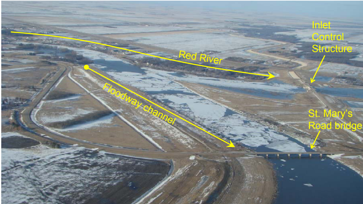
Figure 2. Ice pileup in the area of the Floodway inlet and the Red River leading into Winnipeg in the spring of 2009.
