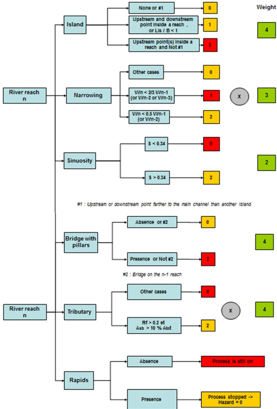
Figure 4 : Adjusted conceptual model. The green squares are the relative weight gives to each parameter except the rapids: island (4), narrowing (3), sinuosity (2), bridge with pillars (4), tributary (4). The red squares represent values taken in a case study. Here the ice jam predisposition index IJPJ gives  $19 / 34 = 0.56$ .
