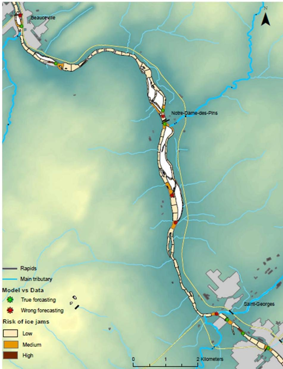
Figure 3 : First results of the model for a 30 km river reach the Chaudière River. The low risk segments are in pale yellow, the medium risk segments are in orange and the only high risk segment is in brown. According with validation data, the areas that were correctly forecasted appear in green stars (7) and those incorrectly forecasted appear in red stars (5).
