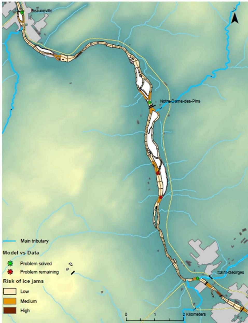
Figure 5 : Improved results for the same 30 km river reach of the Chaudière River (Figure 2) The adjusted conceptual model solves the problem for three segments incorrectly forecasted by the initial version of the model (green stars). However, the wrong detection remains for two segments over the five areas previously incorrectly forecasted. Further, there are more medium risk segments (orange) of ice jams with the adjusted model but no high risk segment (brown).
