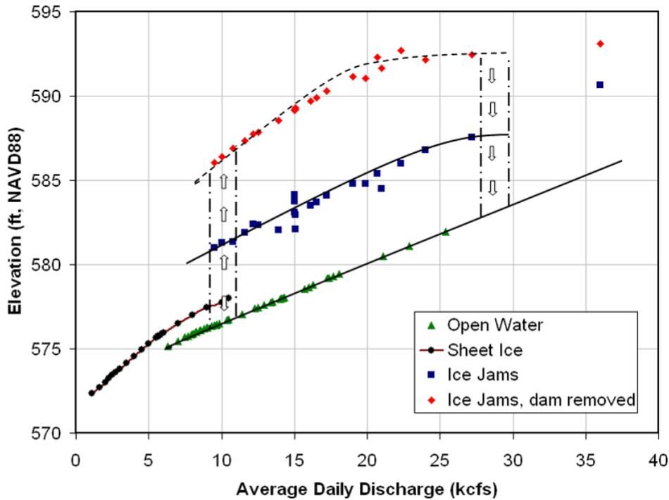
Figure 4. Ice Affect Stage Discharge at State Street, with and without Dam.
