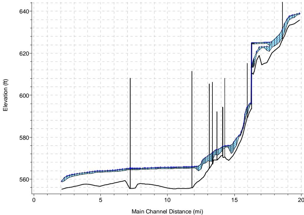
Figure 3. Freezeup Ice Profile, 1959. Upper profile is with dam in place, lower profile is with dam removed, ice shown in hatched blue.
