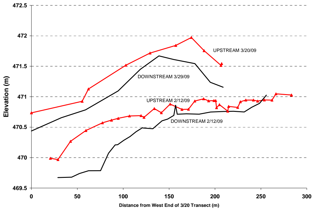
Figure 6. Surface elevations of transects on 2/12/09 and 3/20/09
