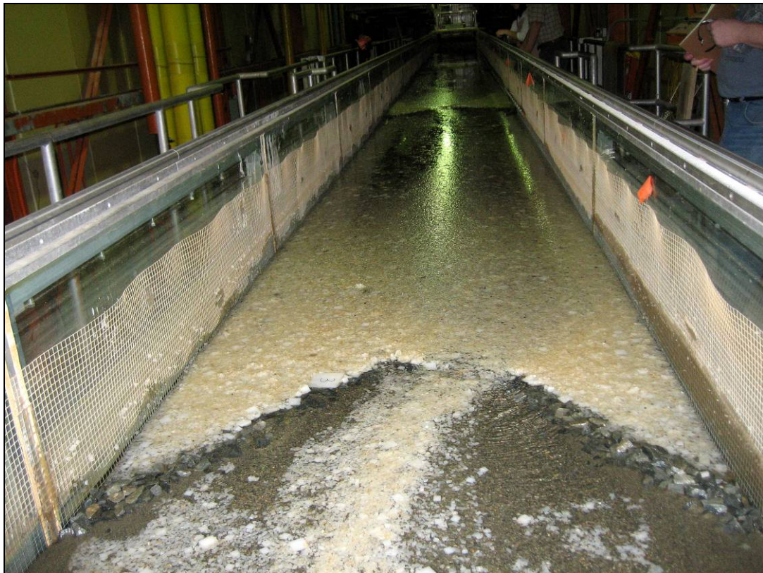
Fig. 4. Near ice stoppage at cross-vanes during physical model testing in CRREL Flume.
