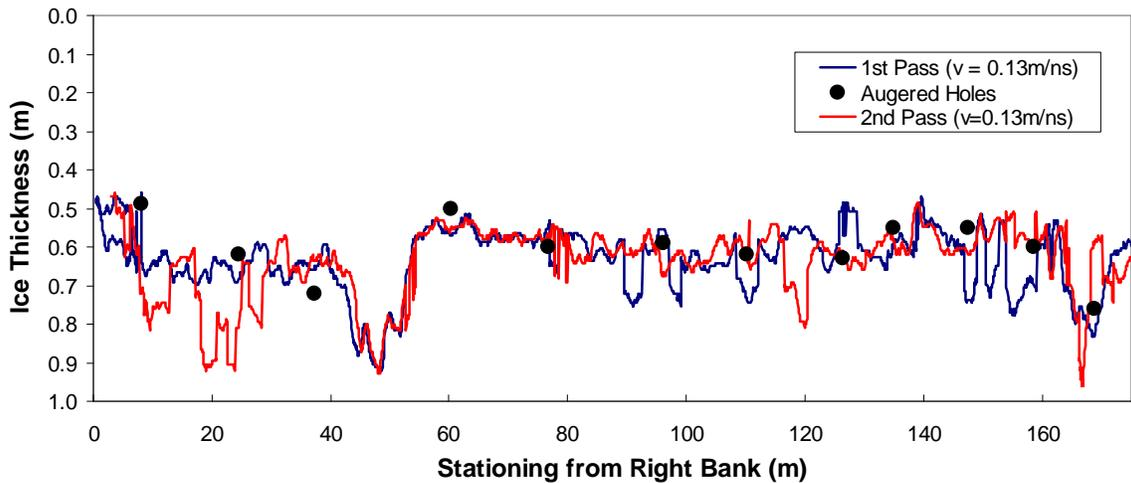
Figure 2: Ground based data collection using 400 MHz antenna on cross section 2.
