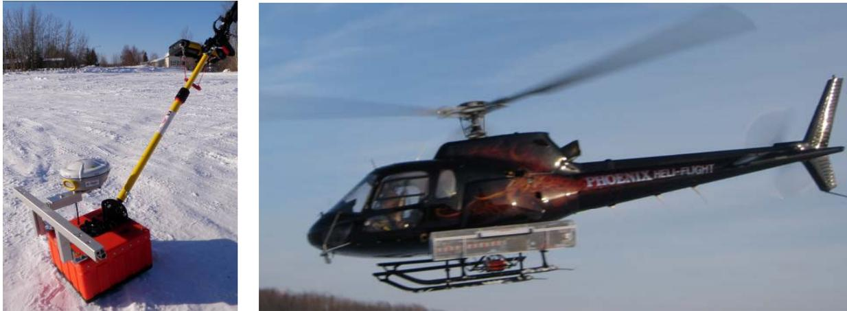
Figure 1: Conventional ground based and aerial GPR data collection via helicopter.
