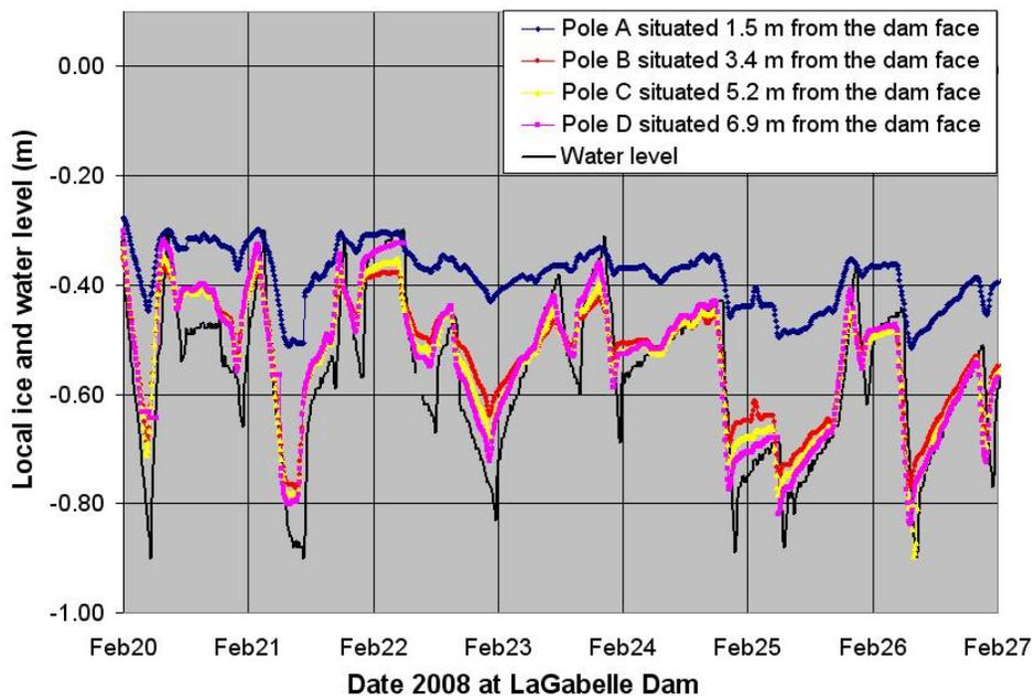
Figure 4 - Poles vertical displacement and water level fluctuation
