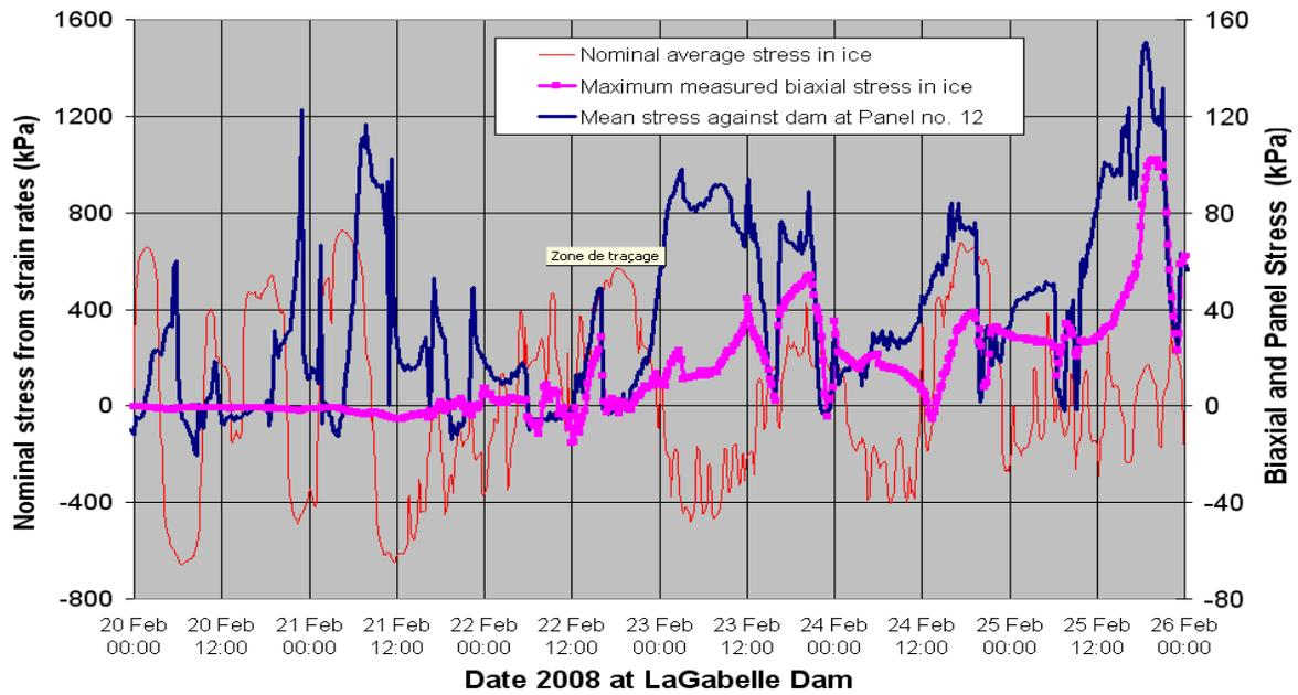
Figure 9. Comparison of stresses in the ice (from strain rates and biaxial gauges) and against dam face (at panel no. 12)
