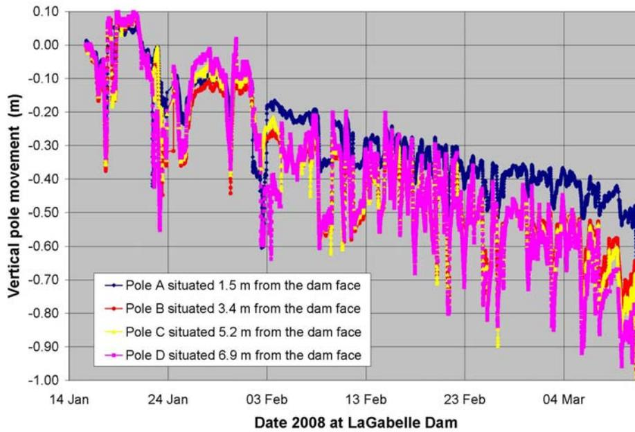
Figure 5. Vertical movement of poles from January to March 2008
