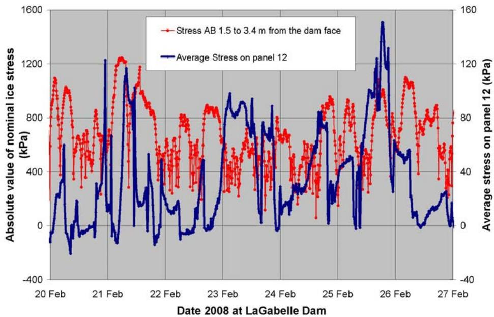
Figure 8 – Stress between adjacent poles and average stress measured at Panel no. 12
