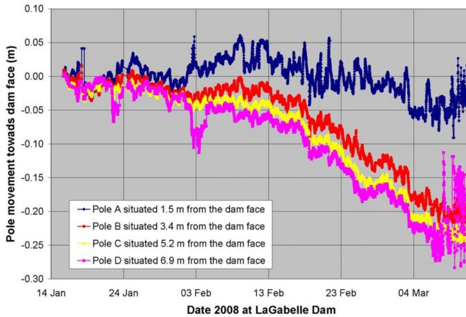
Figure 6 - Lateral displacement of ice sheet
