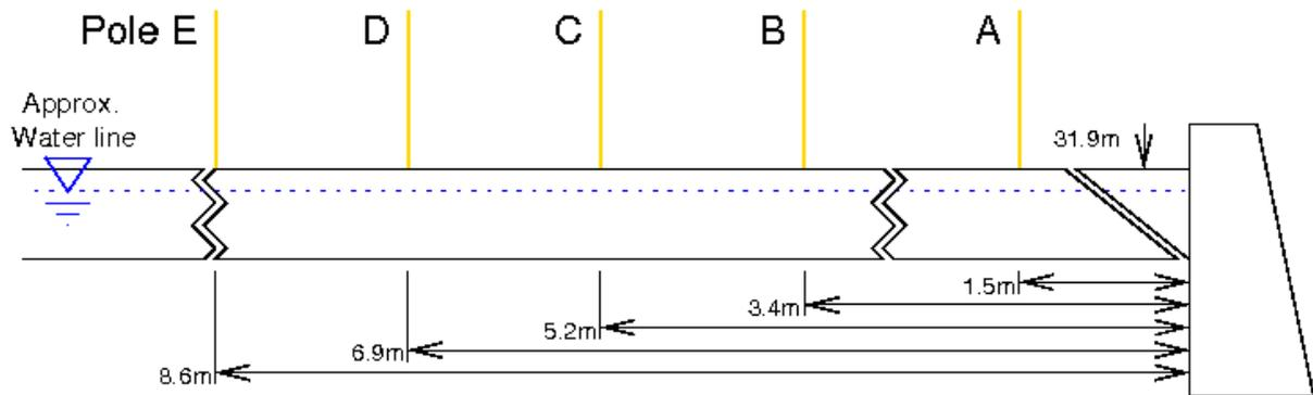
Figure 2. Location of poles placed in the ice perpendicular to dam face
