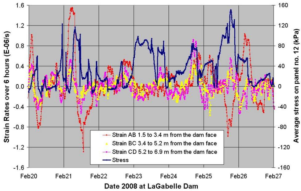
Figure 7 – Strain rate between poles and measured maximum stress against dam face
