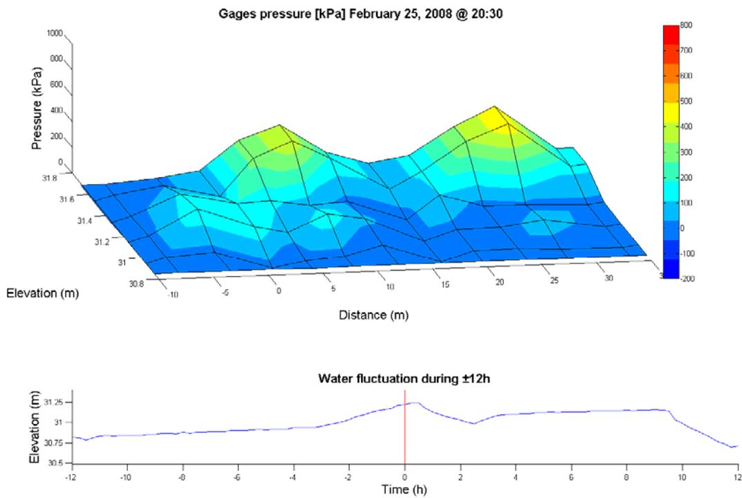
Figure 10 - Three dimensional snapshot of ice stress on dam
