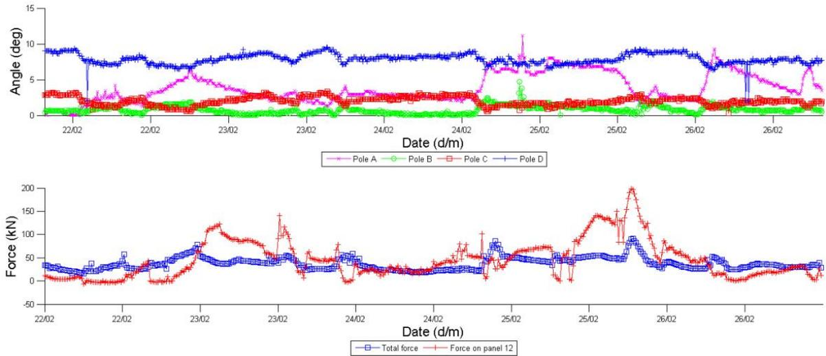
Figure 3. Rotation of poles and resulting force on dam (opposite poles at panel no. 12 at X = 5 m) and total average force from 12 panels (from X = -5 to 37 m)
