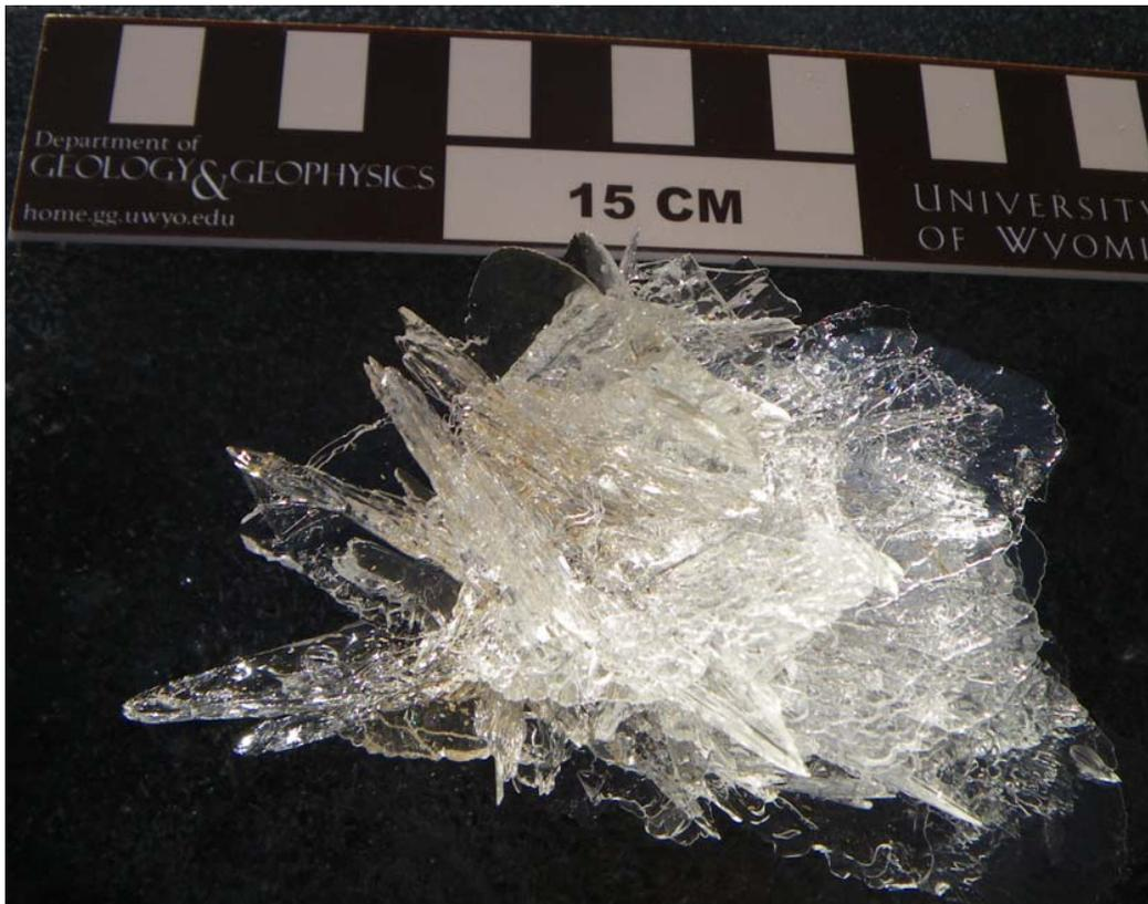
Figure 1. Laramie River anchor ice sample; the largest, blade-shaped ice crystals are 5cm long.
