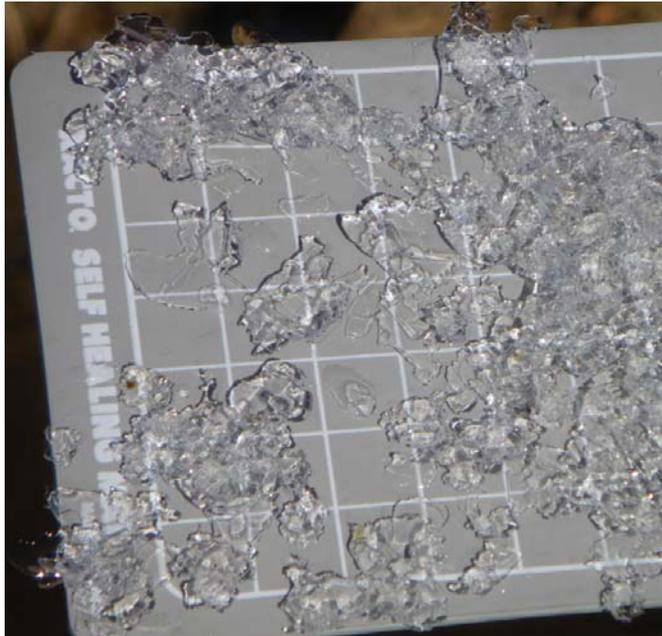
Figure 3. Disaggregated frazil crystals on a plastic grid. Note irregular, 2 cm diameter bladed ice crystal in left center of photograph. Grid spacing is 1.27 cm.
