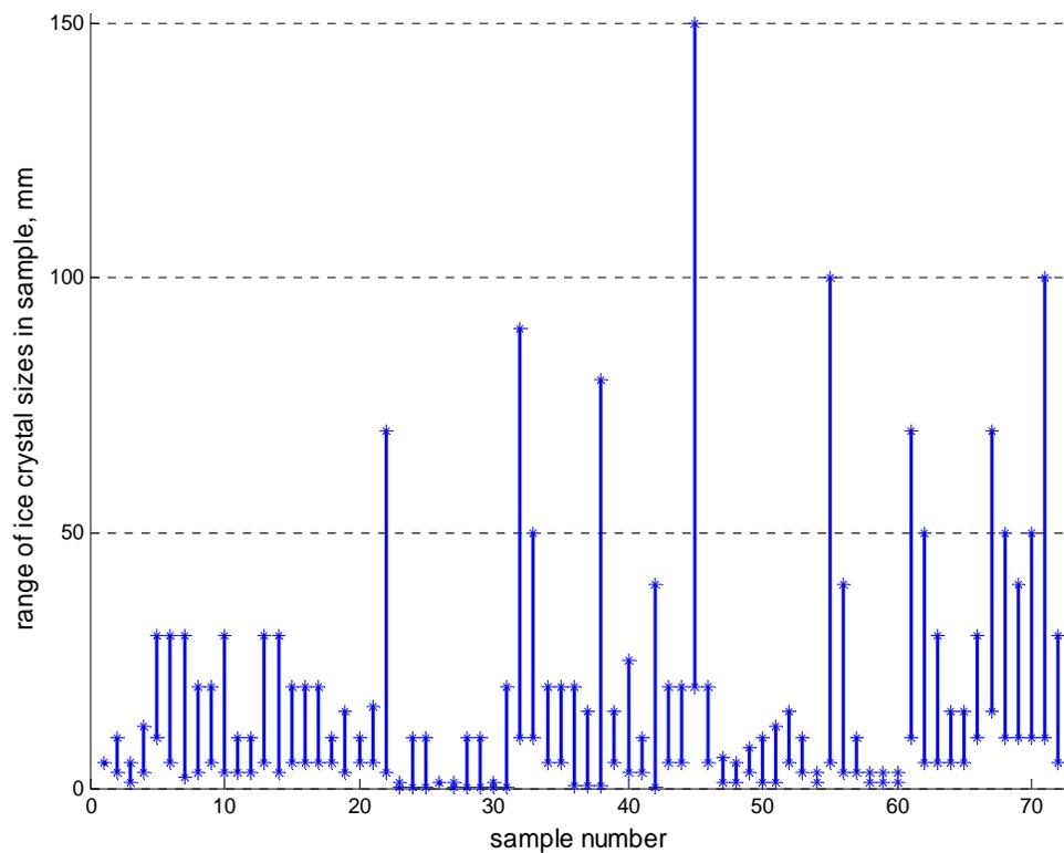
Figure 4. Range of individual ice crystal sizes collected from Laramie River anchor ice masses during fall 2008
