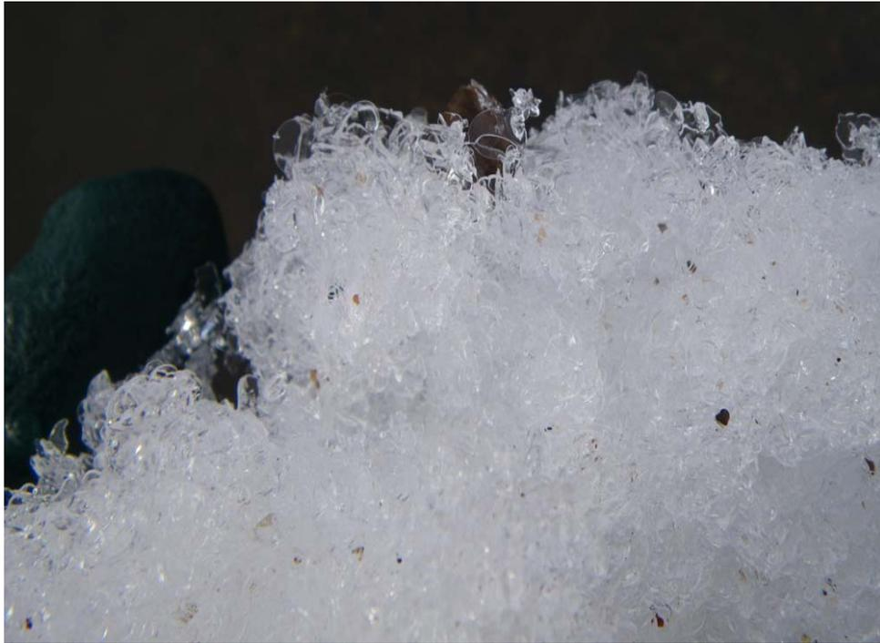
Figure 5. Disc-shaped frazil crystals incorporated into a Laramie River anchor ice mass. The striking frazil crystal in the upper left center of the image is 5mm in diameter. Although several frazil discs are visible on the edge of the anchor ice mass, ice crystals in the interior of the mass have grown into irregular shapes.
