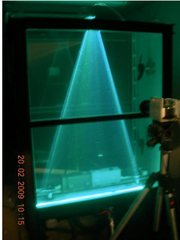
**Figure 3:** Experimental setup using a laser sheet for lighting.
