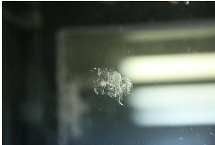
**Figure 7:** Picture of a suspended frazil ice floc using an SLR camera.
