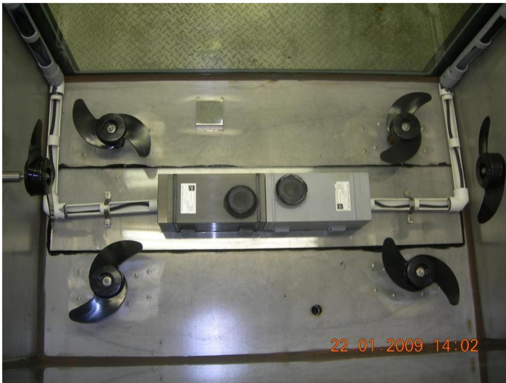
**Figure 2:** Top view of the frazil ice tank setup showing the high and low frequency SWIPS, the Plexiglas base plate, and cables inside the hollow PVC tubes; two of the side mounted propellers and the four bottom mounted propellers are also shown.
