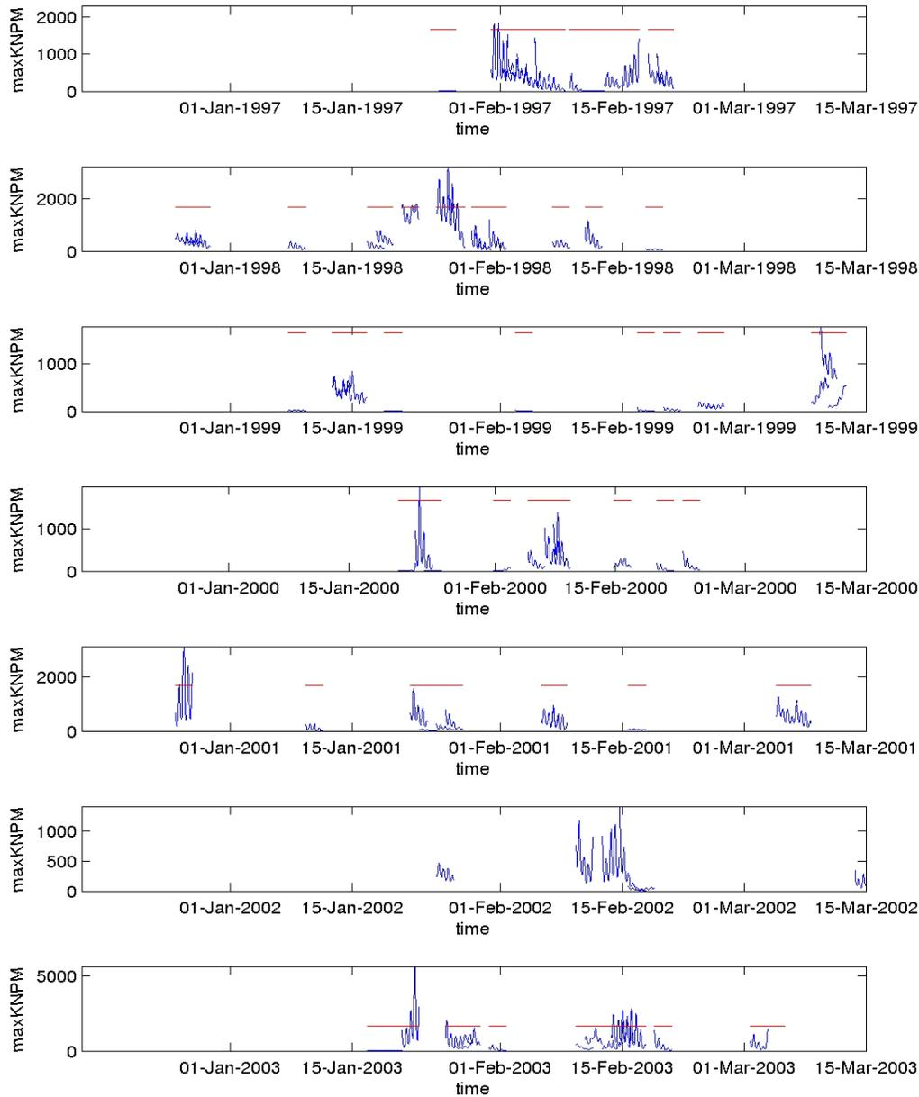
Figure 5.1: Blended time series of the 7 years of ice line load event data (pressure x mean ice thickness) for the terminal site, with the “significant event threshold” of 1.67 kN/m shown by the horizontal red lines. Only the last 48 hours of each simulation run are plotted here.
