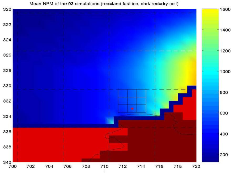
**Figure 5.5:** A map of the region around the proposed Gros-Cacouna terminal site, with the land shown in dark red, the fast ice in red, and the coastline by the black line. The mean ice pressure value (expressed as the ice line load in Nm-1) is depicted here. The pressure values are averaged over the 93 simulations, and cover the 7 winter periods from February 1997 to March 2003. The red dot indicate the location of the terminal site.
