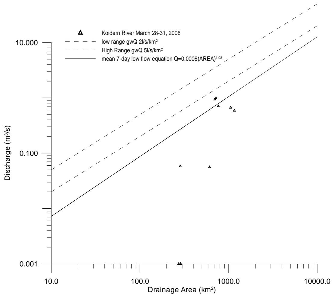
**Figure 4:** Koidern River discharge measurements against drainage area. The dashed lines represent the expected range of groundwater discharge (Williams and van Everdingen, 1973) and the solid line shows the 7-day low-flow equation (Janowicz, 1991). Zero flow is plotted as 0.001 m<sup>3</sup>/s
