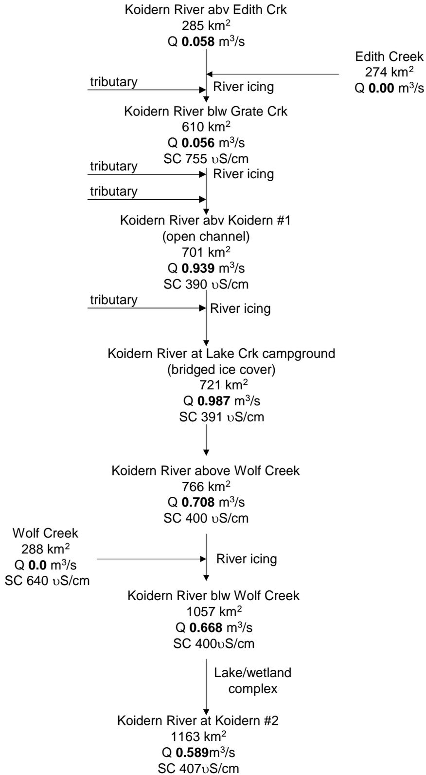
**Figure 3:** Schematic showing the survey cross-sections relative to the main stem, drainage area, discharge, and specific conductance
