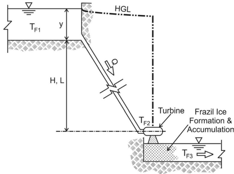
Figure 5. Frazil formation and accumulation within a turbine and its outlet; freezing temperatures  $T_{F1} = T_{F3} = 0.00^{\circ}\text{C}$ ;  $T_{F2} < 0.00^{\circ}\text{C}$
