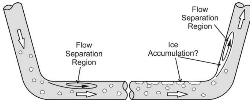
Figure 8. Flow separation at the base of an inverted siphon, and flow along the base may increase ice accumulation
