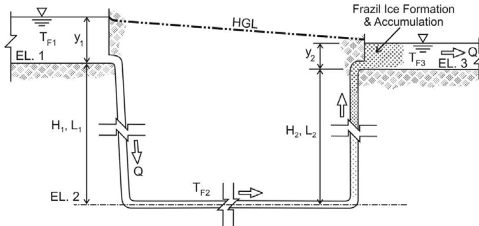
Figure 7. Frazil formation in an inverted siphon;  $T_{F1} = T_{F3} = 0.00^{\circ}\text{C}$ ;  $T_{F2} < 0.00^{\circ}\text{C}$
