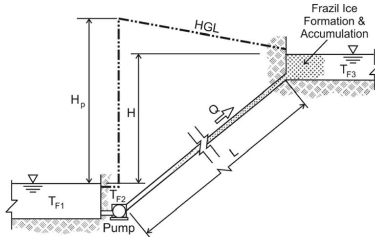
Figure 6. Frazil formation in a pump-line pipe:  $T_{F1} = T_{F3} = 0.00^{\circ}\text{C}$ ;  $T_{F2} < 0.00^{\circ}\text{C}$
