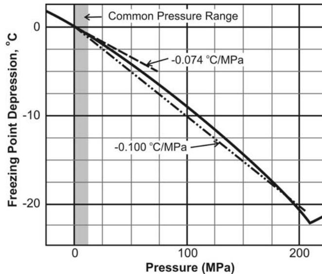
Figure 3. A portion of the relationship between freezing-point depression,  $\Delta T_F$  and absolute pressure for water; common pressure range for hydraulic structures is indicated
