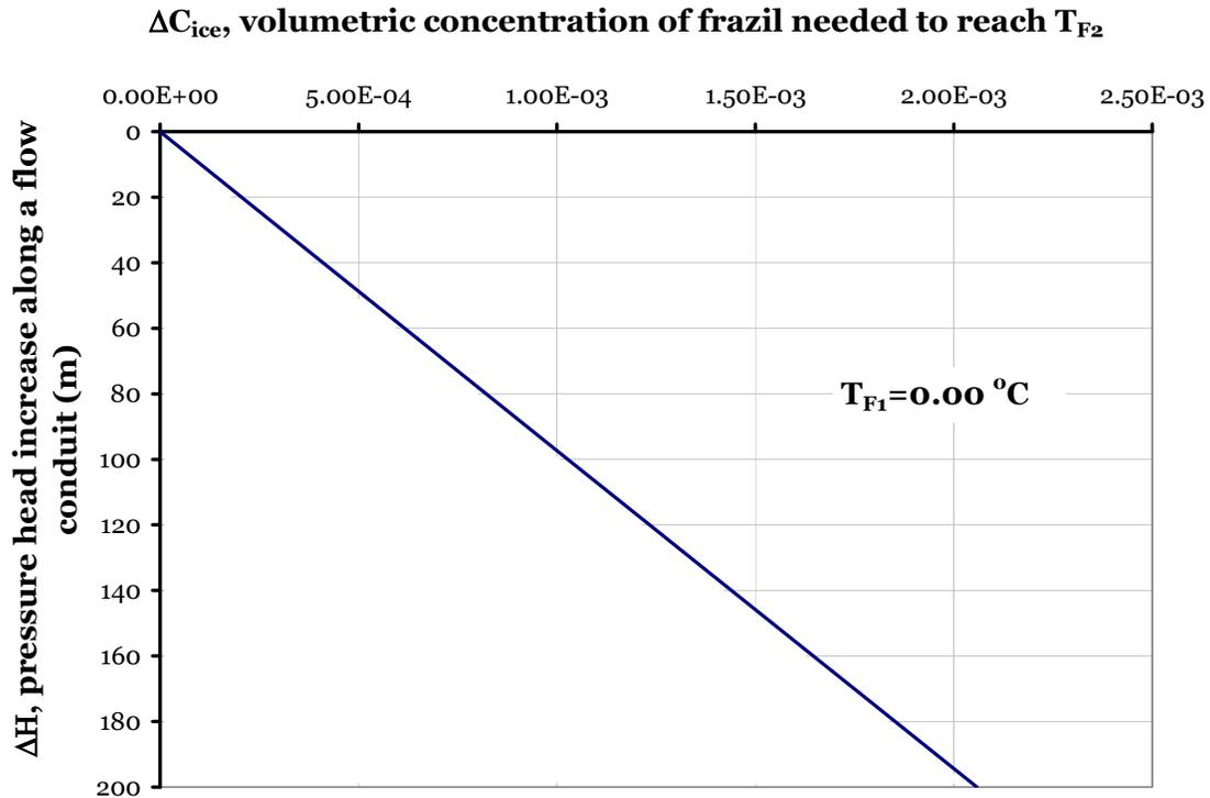
Figure 4. Variation of frazil concentration needed to reach final freezing temperature ( $T_{F2}$ ) as a function of pressure-head increase (or elevation drop) along a conveyance structure; initial freezing temperature is  $T_{F1}$
