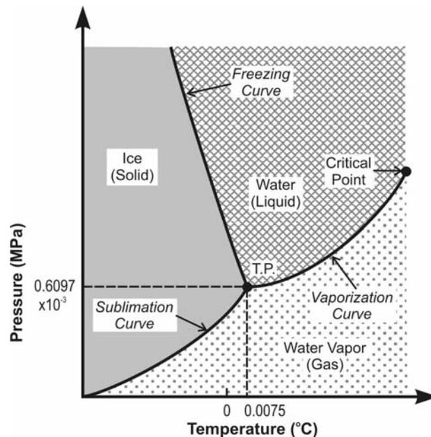
Figure 2. A portion of the phase diagram of water (T.P. is the triple point for water)
