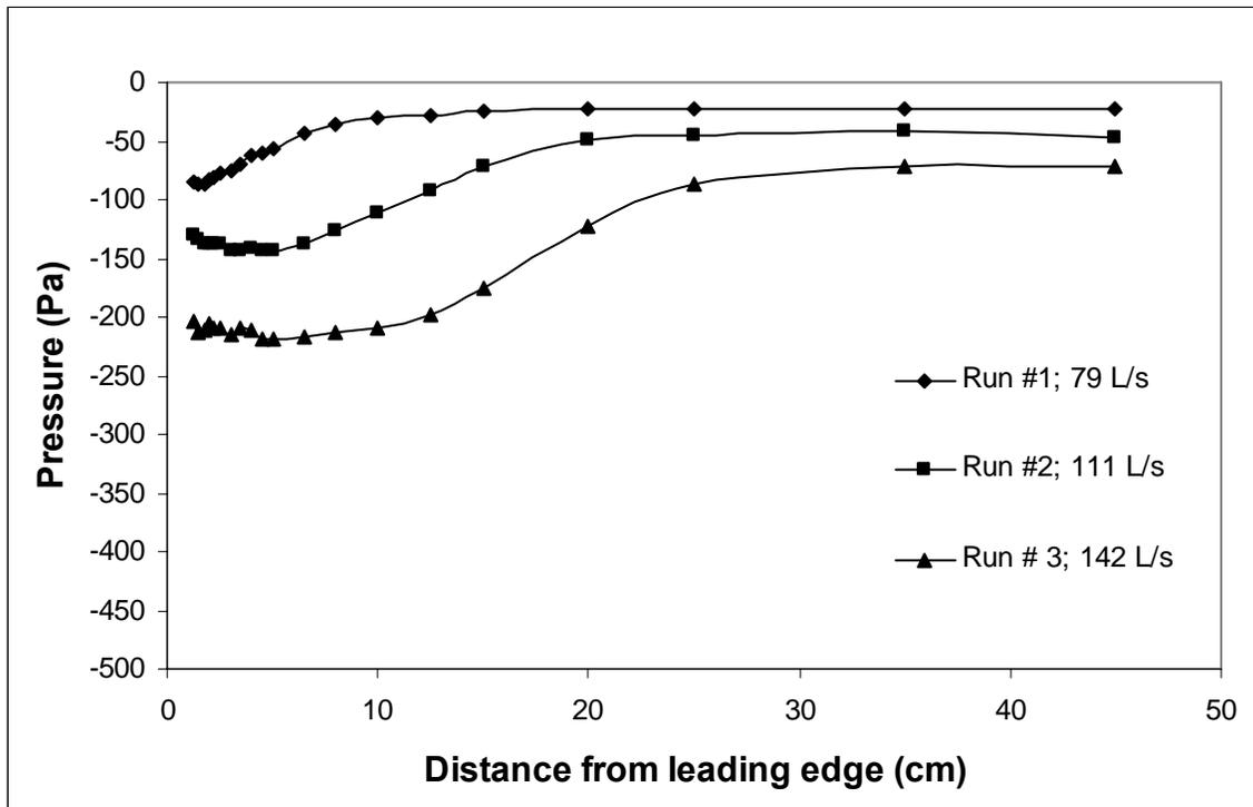
Figure 5. Dynamic pressures measured under the ice block for  $t = 3.35 \text{ cm}$ ,  $H = 30.2 \text{ cm}$  ( $t/H = 0.11$ ).
