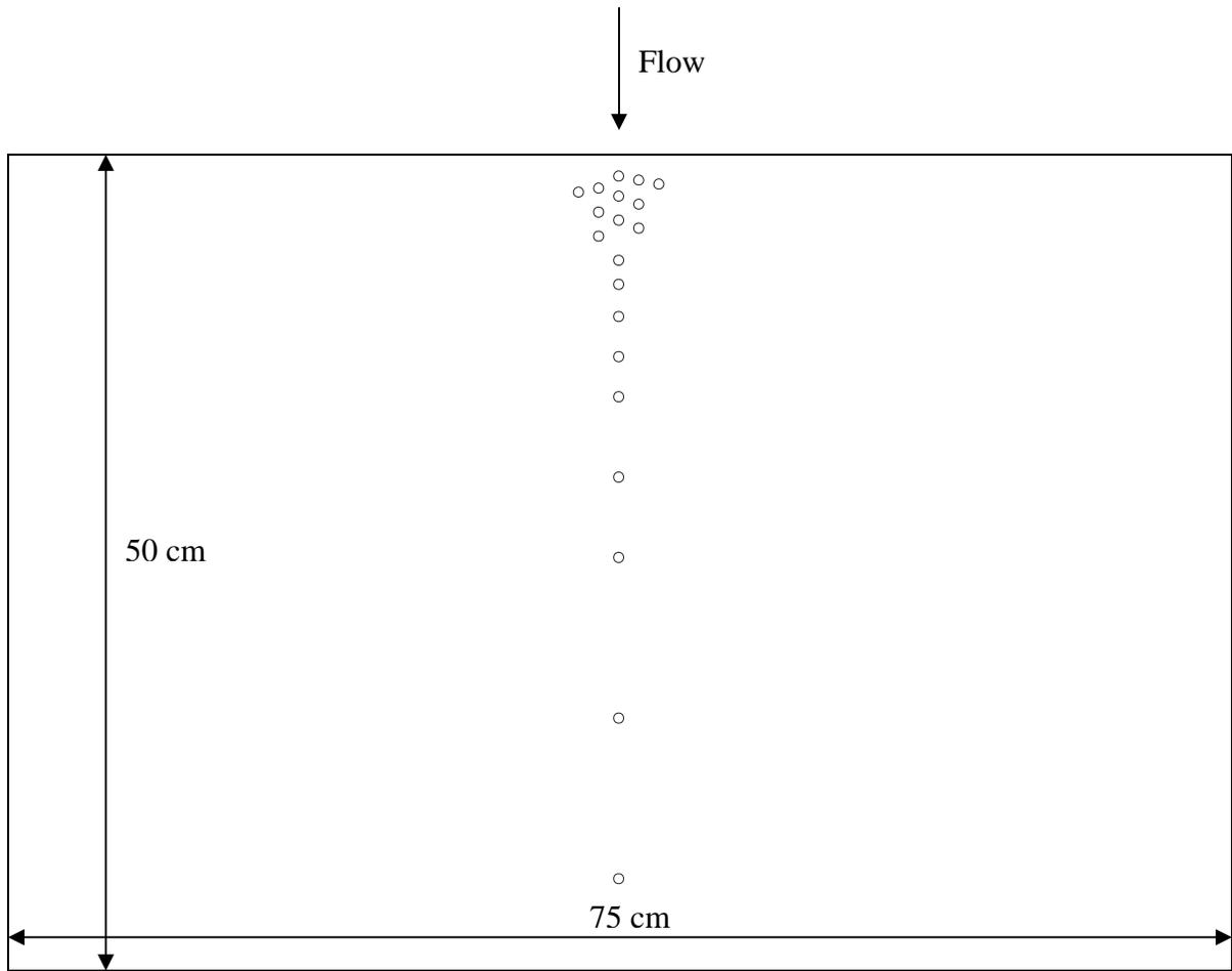
**Figure 3. Locations of pressure taps in ice block.**
