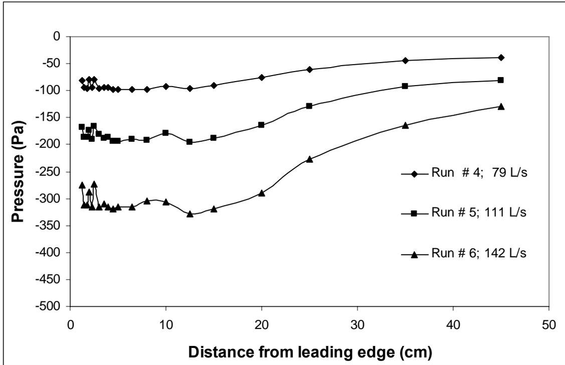
Figure 6. Dynamic pressures measured under the ice block for  $t = 6.02$  cm,  $H = 30.03$  cm ( $t/H = 0.20$ ).
