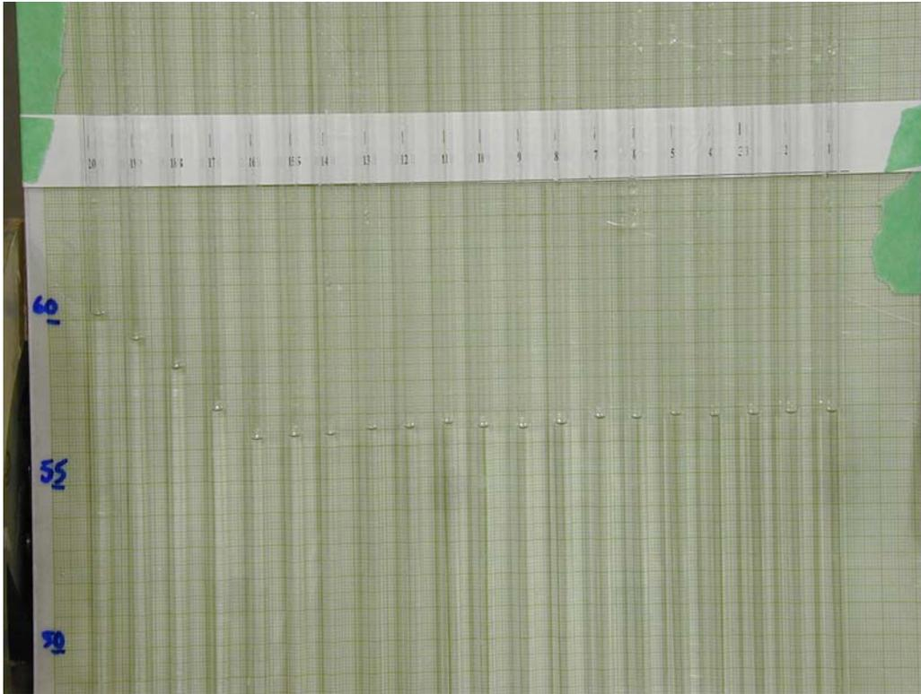
Figure 4. Manometer board for  $Q = 111 \text{ L/s}$  and  $t/H = 0.2$ .
