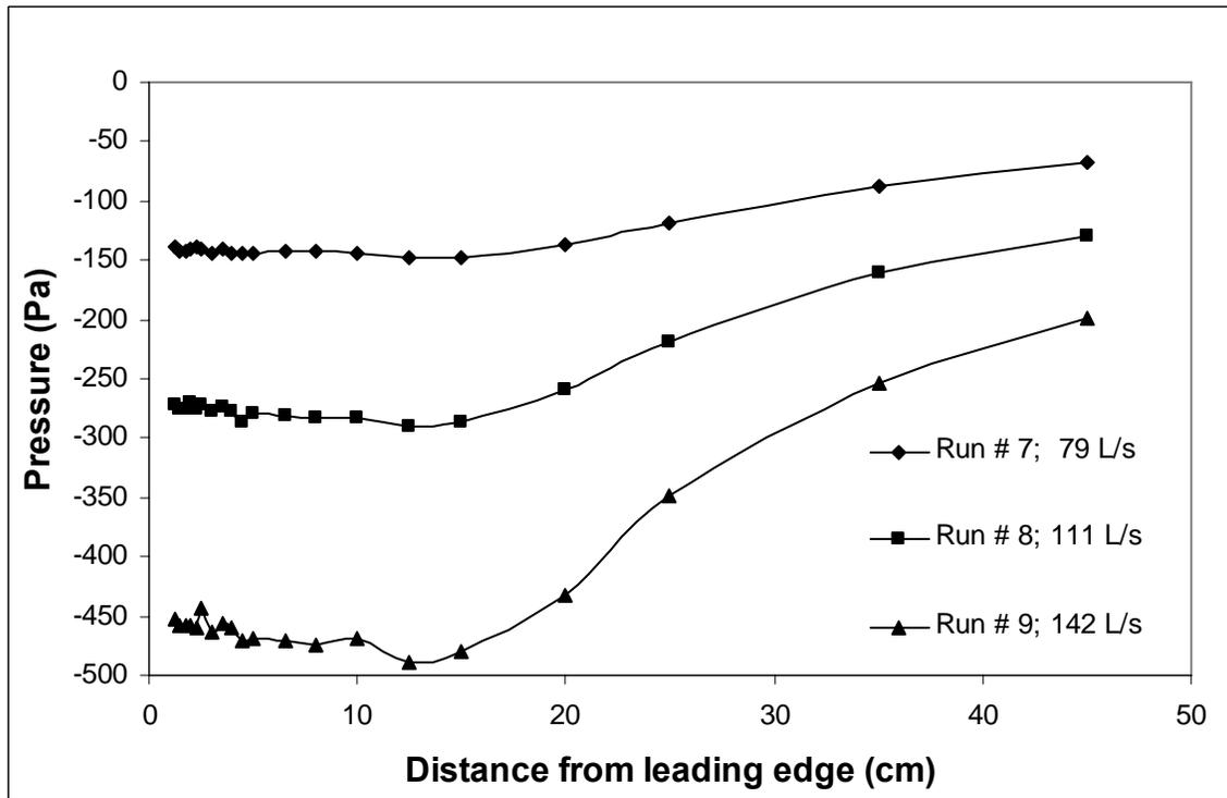
Figure 7. Dynamic pressures measured under the ice block for  $t = 8.39$  cm,  $H = 29.02$  cm ( $t/H = 0.29$ ).
