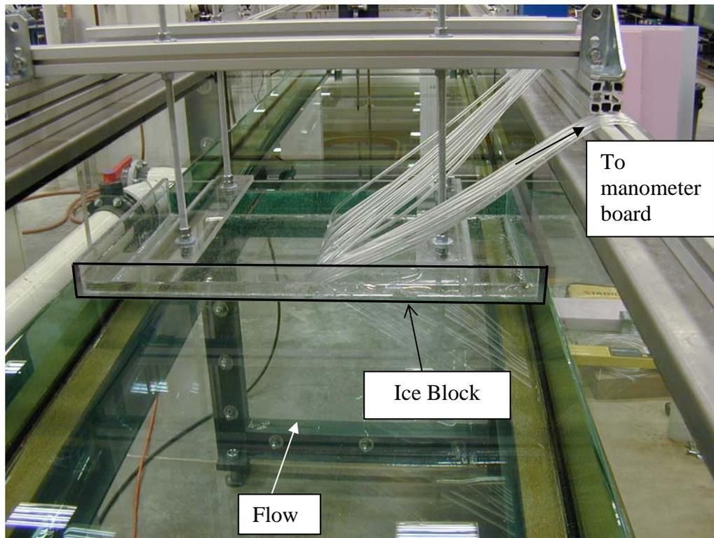
Figure 2. Experimental flume - Ice block setup, looking downstream.
