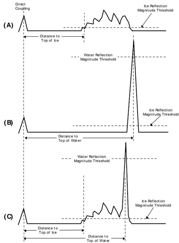
*Fig. 8 – Decision thresholds and range determination. (A) Radar signal reflected from dense icepack. (B) Radar signal reflected from open water. (C) Radar signal reflected from sparse icepack.*
