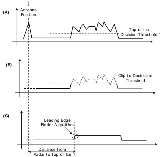
Fig. 10 – Determination of the distance from radar antenna to top of ice. (A) Raw radar signal showing top of ice decision threshold level. (B) Clipped signal. (C) Leading edge detector for locating top of icepack.
