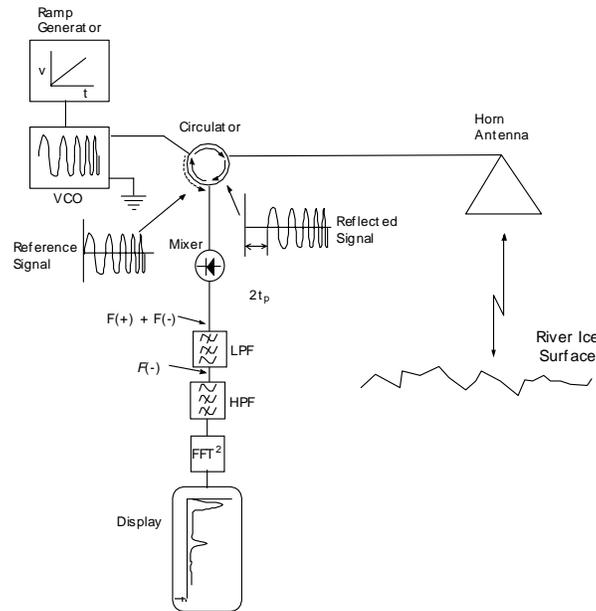
Fig. 3 – Block diagram of a FM-CW radar system.
