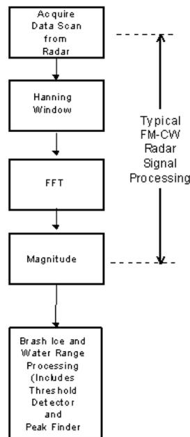
*Fig. 7 – Radar signal processing block diagram.*
