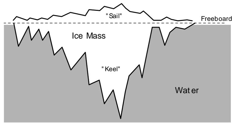
*Fig 2 – Representation of components of a floating mass of ice.*
