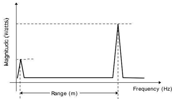
*Fig. 4 – Arbitrary power spectrum illustrating radar signal magnitude and the relationship between range and frequency for an FM-CW radar where range (m) is directly proportional to frequency (Hz).*
