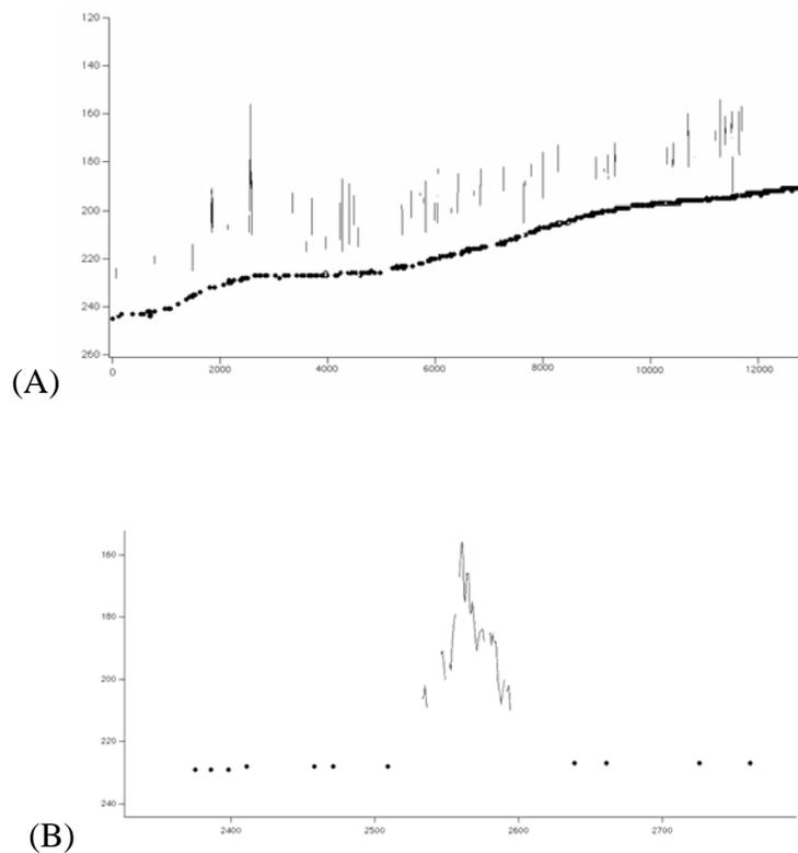
*Fig. 15 -- Output data from Ice Thickness Measuring Radar System for a Sparse Ice Cover. Top graph (A) shows an extended time profile and lower graph (B) shows an expanded view of a shorter time segment. Line on graphs represent profile of brash ice sail. Dots on graph*
