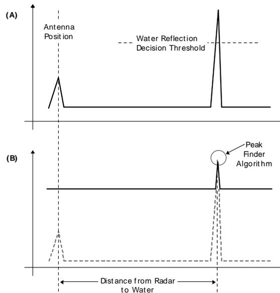
Fig. 11 – Determination of the distance from the radar antenna to the water surface. (A) Raw radar signal showing water reflection threshold. (B) Clipped radar signal for water surface range detection.
