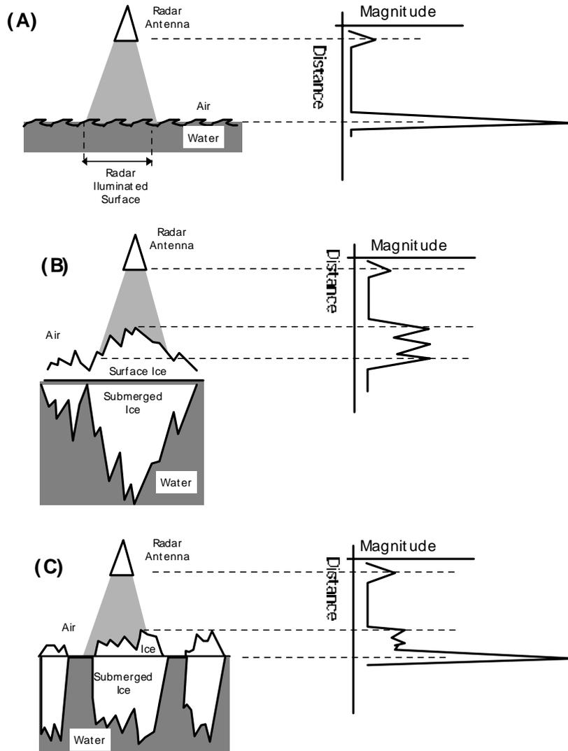
*Fig. 6 – Typical radar waveforms for a variety of ice and water conditions. (A) Radar reflection from open water surface. (B) Radar reflection from dense brash ice. (C) Radar reflection from sparse brash ice.*
