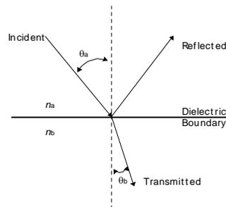
*Fig. 5 – Illustration of reflection and transmission at a dielectric boundary. At an interface of two different dielectric materials, a fraction of the incident radar signal is reflected at the boundary and a fraction is transmitted through the boundary.*
