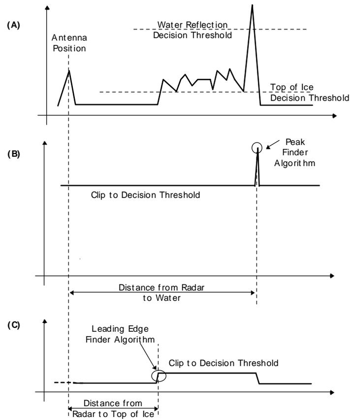
*Fig. 9 – Determination of distance from radar antenna to the top of the ice and the water surface. (A) Raw radar signal showing amplitude thresholds. (B) Radar signal clipped at decision threshold for water reflection peak detection. (C) Radar signal clipped at decision threshold for top of icepack detection.*
