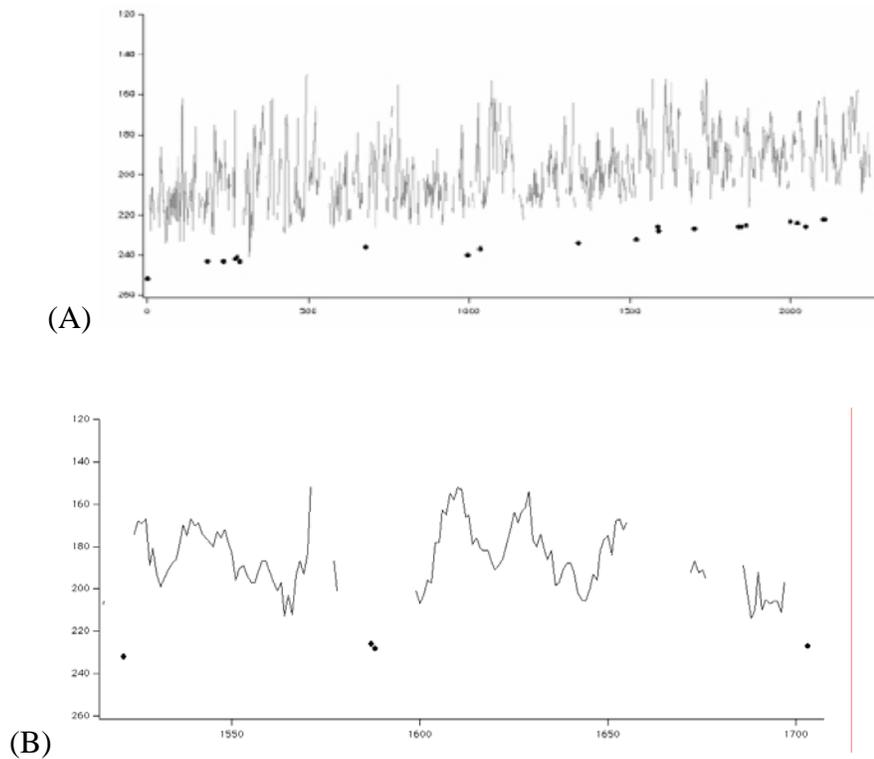
*Fig. 13 – Output data from Ice Thickness Measuring Radar System for a Dense Ice Cover. Top graph (A) shows an extended time profile and lower graph (B) shows an expanded view of a shorter time segment. The line on each graph represents the profile of brash ice sail. Dots on the graphs represent distance from radar antenna to water surface. The vertical axis is centimeters and the horizontal axis is seconds.*
