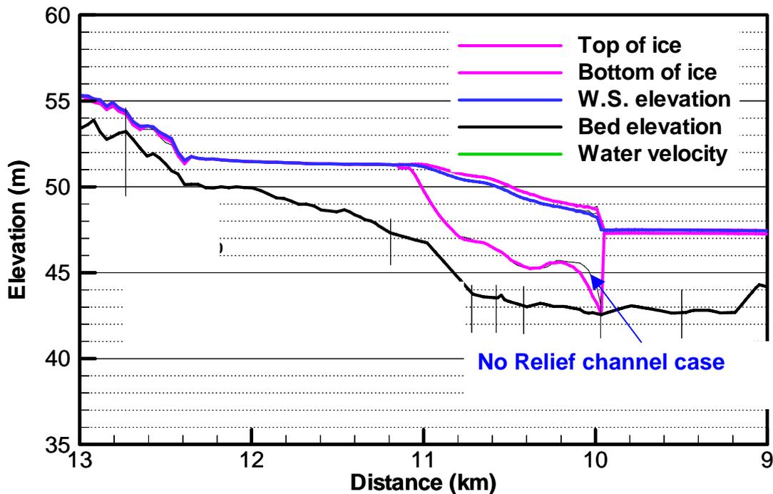
Fig. 3. Ice jam profiles, no-relief channel case compared to 100-m-long relief channel case.
