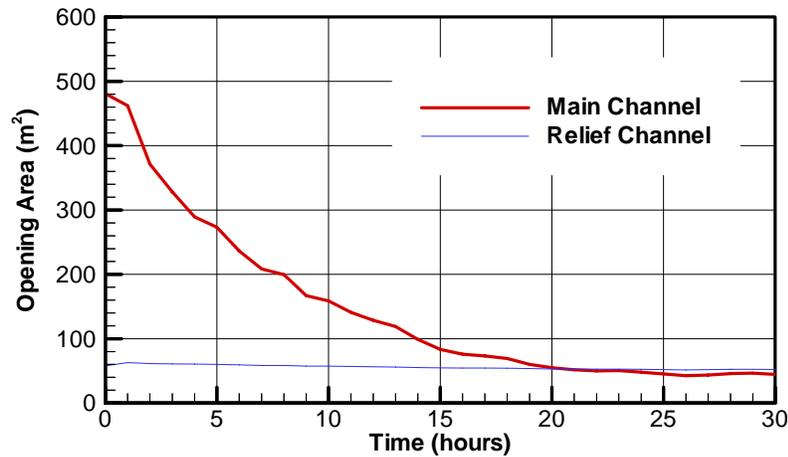
Fig. 8. Under ice water flow areas vs. time for 100-m-long relief channel case.
