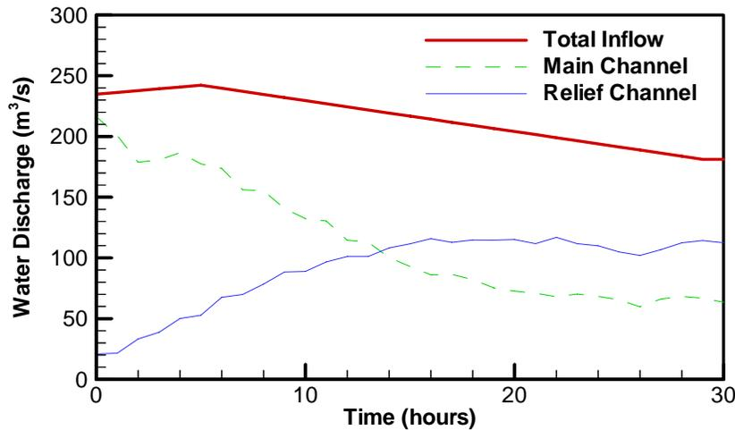
Fig. 9. Water discharge vs. time for 100-m-long relief channel case.
