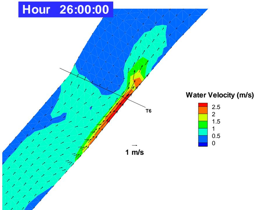
Fig. 7. Water velocity under simulated ice jams, 60-m-long relief channel case (top) compared to 200-m-long relief channel case (bottom).
