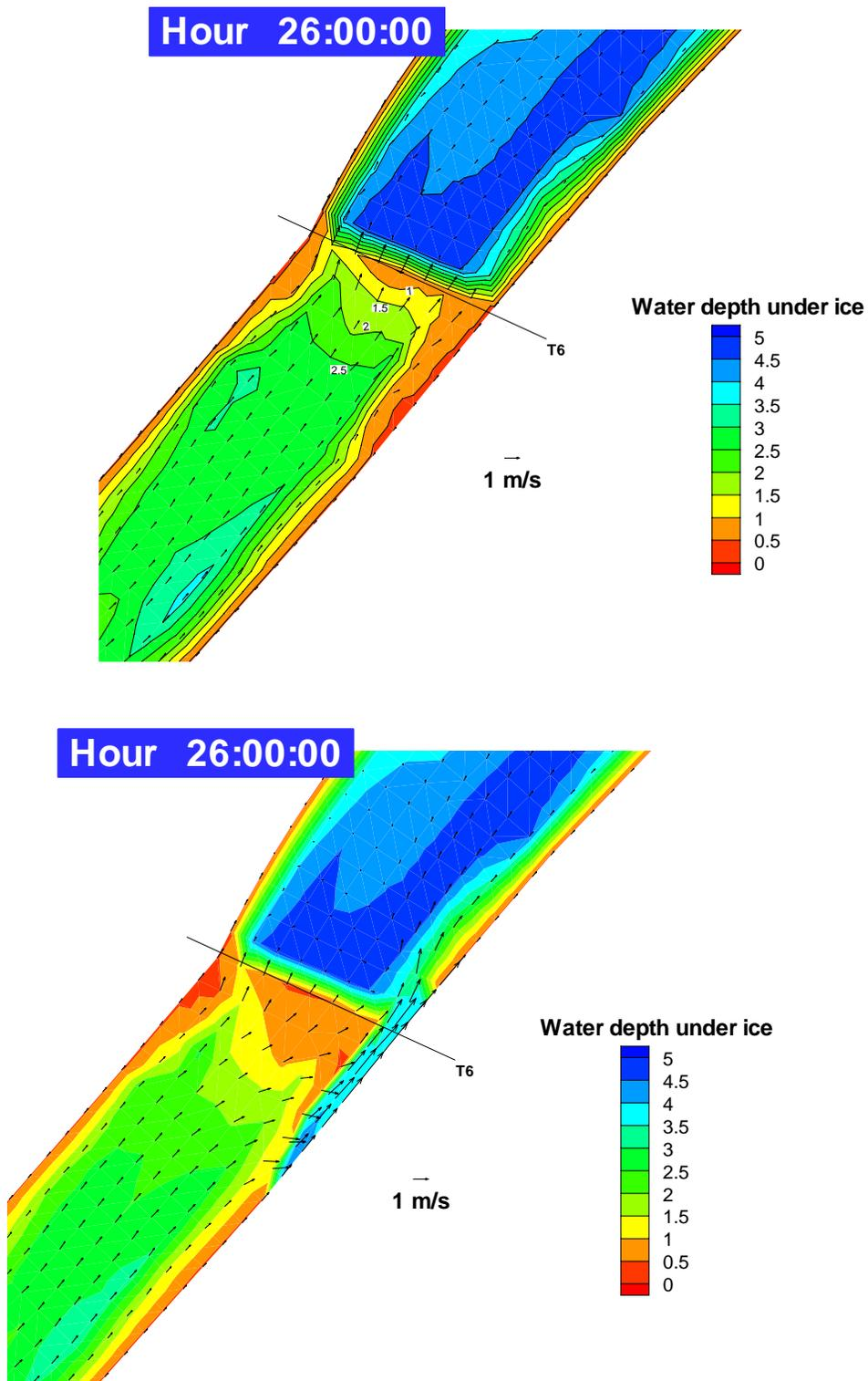
Fig 4. Water depth under simulated ice jams, no-relief channel case (top) compared to 100-m-long relief channel case (bottom).
