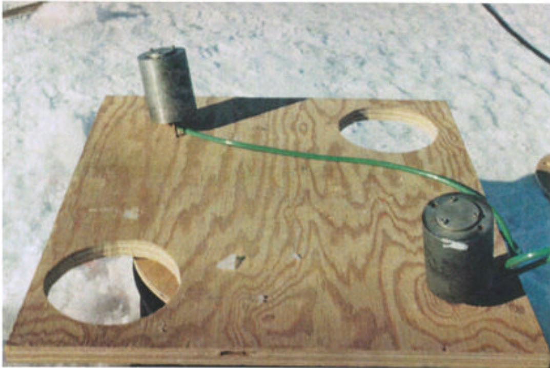
Figure 2: The Geokon stress gages ready for emplacement. Each gage contains two wires 90 degrees apart and the gages are orientated 45 degrees from one another.
