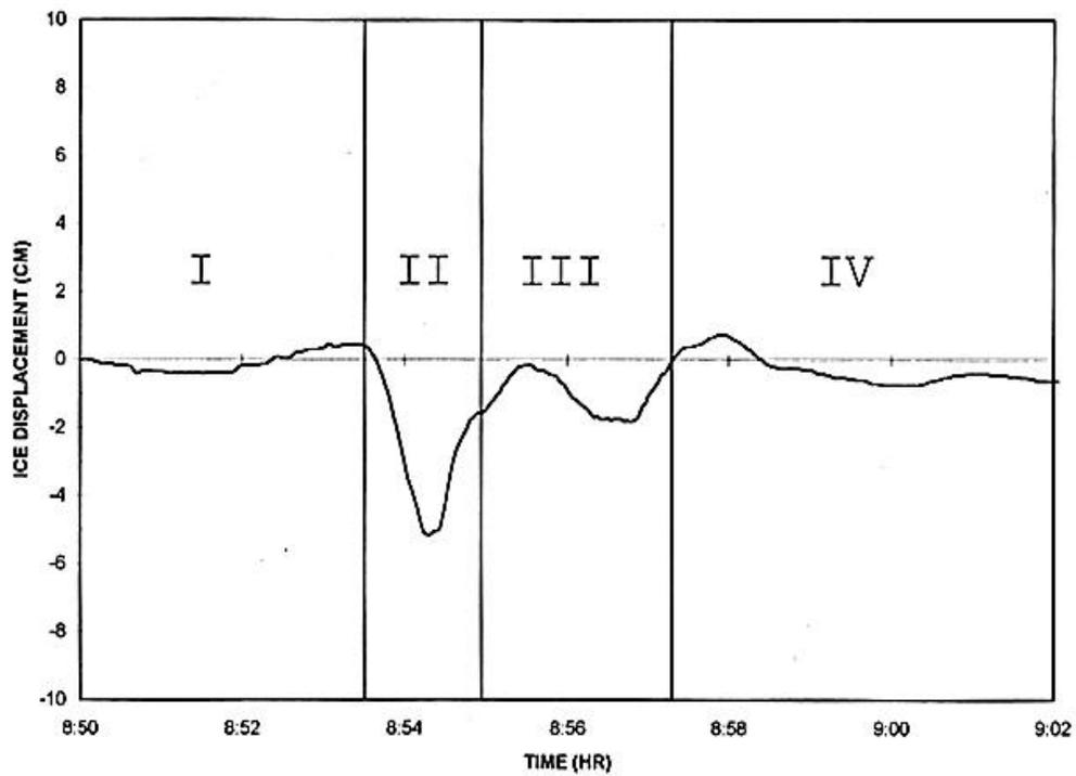
Figure 4: A typical displacement event: in this case the KAPITANAS Gudín, a bulk carrier which was encountered on February 18, 1995.
