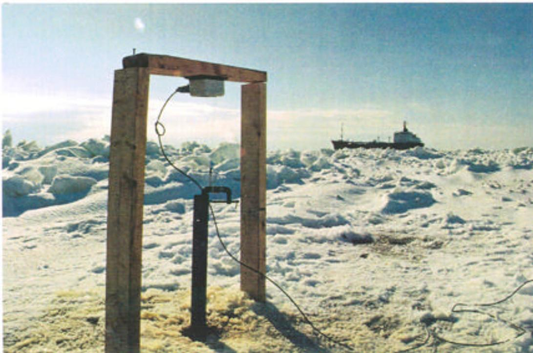
Figure 3: the Endeco wire gage used to measure ice displacement. This gage was placed later in the season and employed a PVC tube to avoid the effect of pressure waves beneath the ice sheet.
