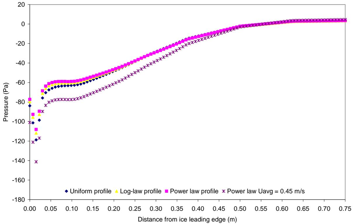
Figure 6: Sensitivity of model results to variation in inlet velocity profile.
