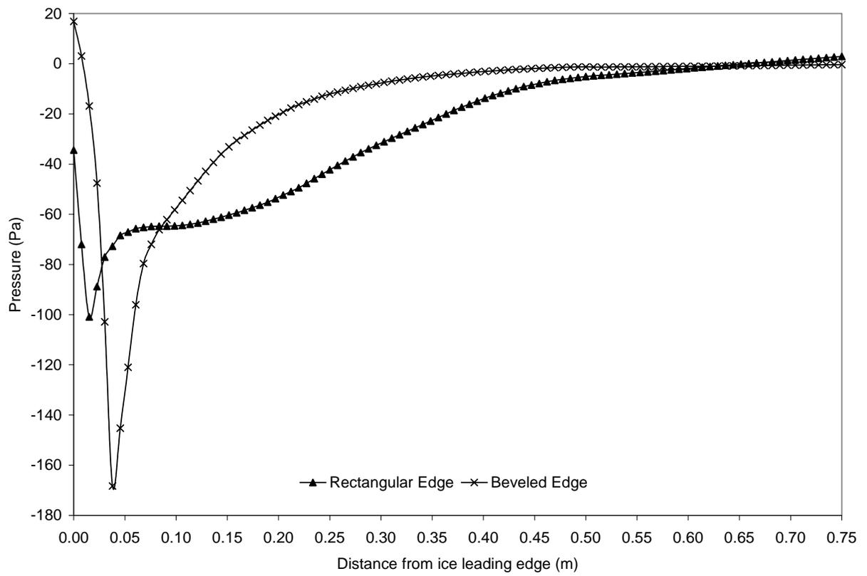
Figure 8: Effect of ice leading edge shape on computed under ice pressure distribution.
