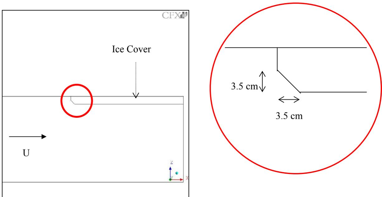
Figure 7: Model configuration for testing a beveled leading edge on the ice cover.
