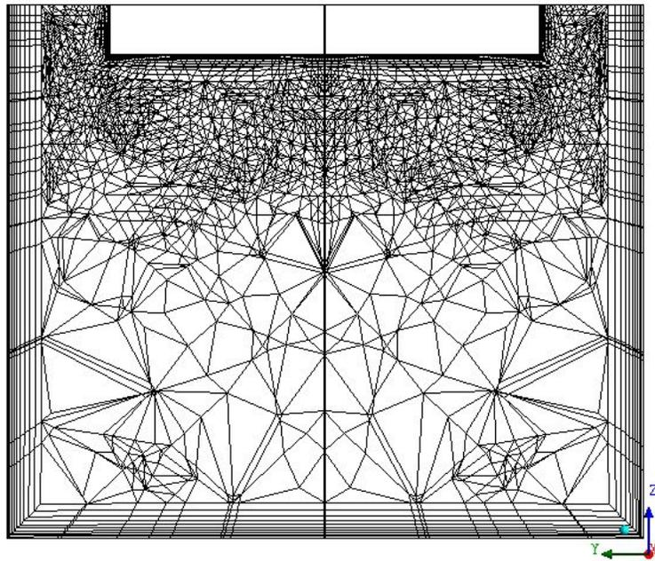
Figure 3. YZ plane at edge of ice cover a) before mesh adaption, and b) after mesh adaption.
