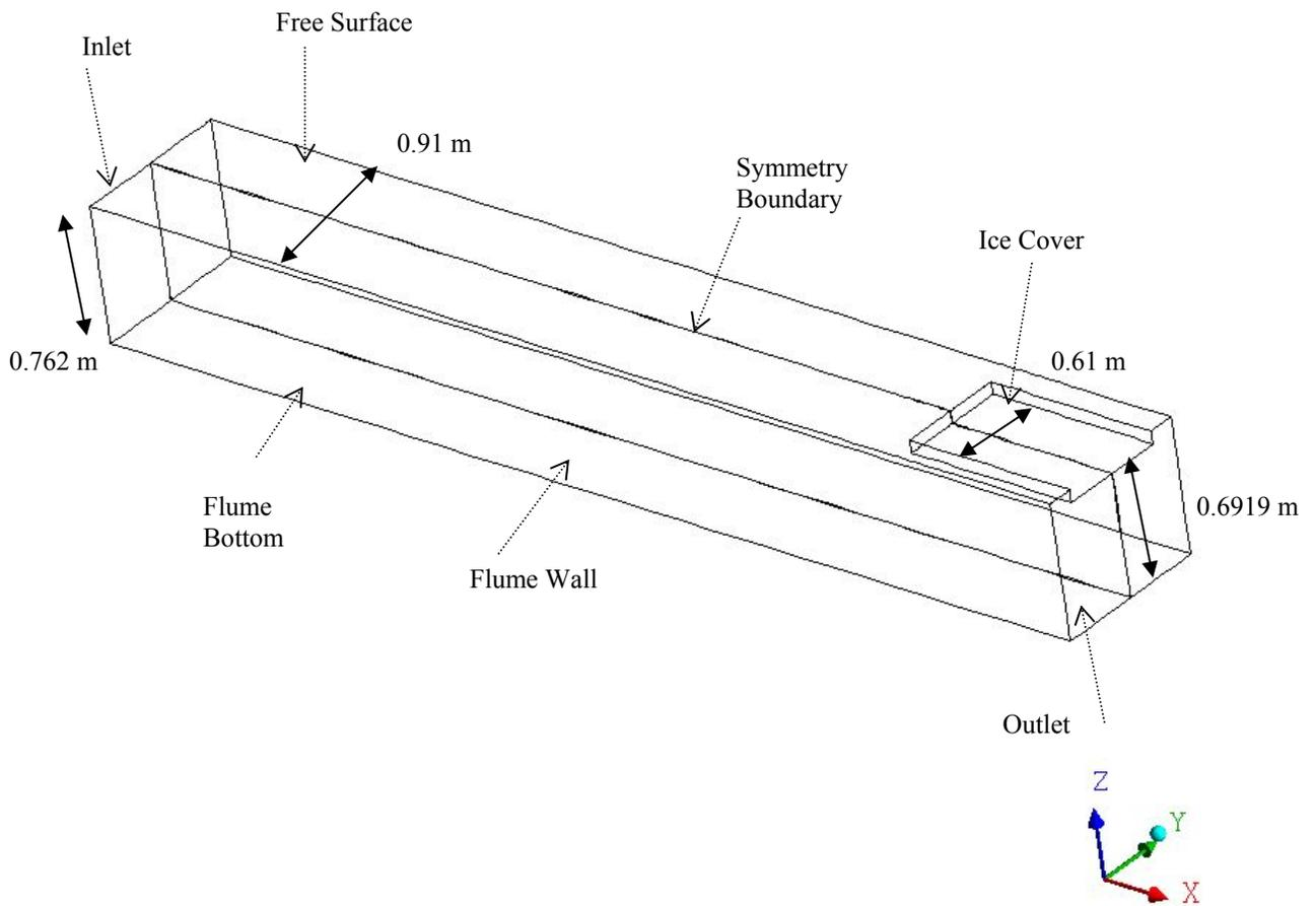
Figure 2: Model geometry for preliminary simulations.
