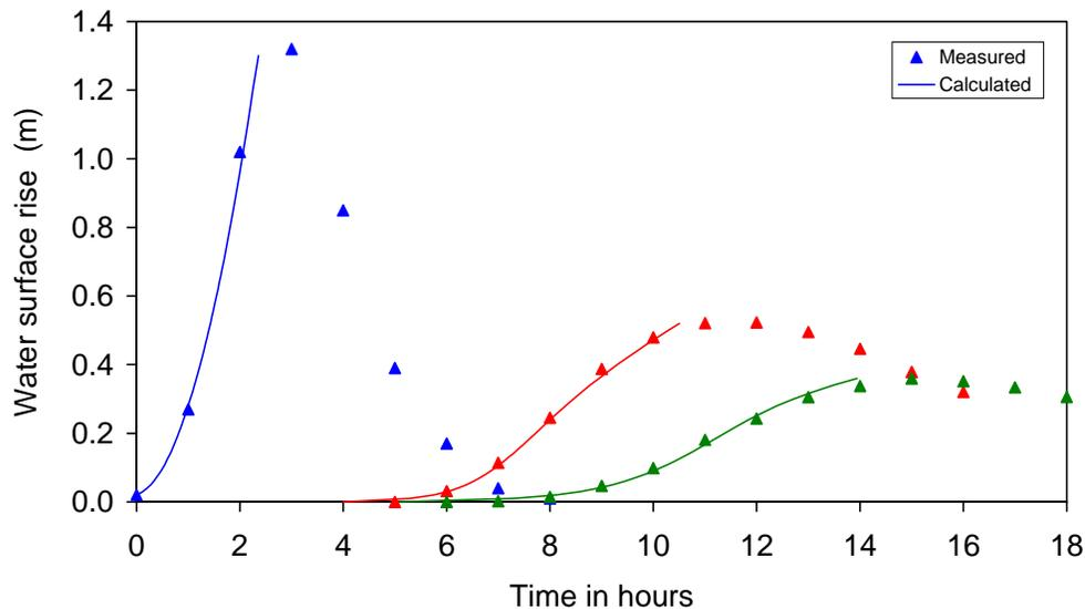
Figure 3. Comparison between measured waves at the three gauging stations and rising-limb portions calculated with the analytical method.
