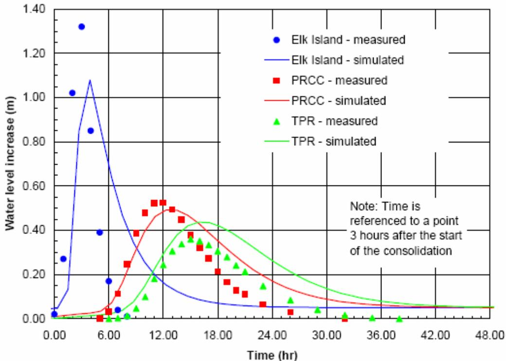
Figure 2. Comparison of measured and simulated stage increases at the three gauge sites downstream of the consolidation area. From Andres et al. (2003).
