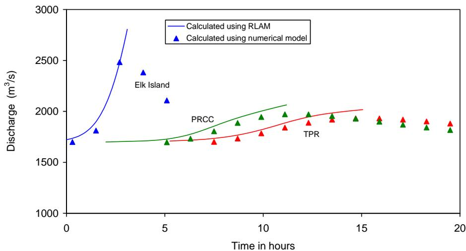
Figure 4. Flow comparisons at the three gauging stations when RLAM is applied to model-generated waves.
