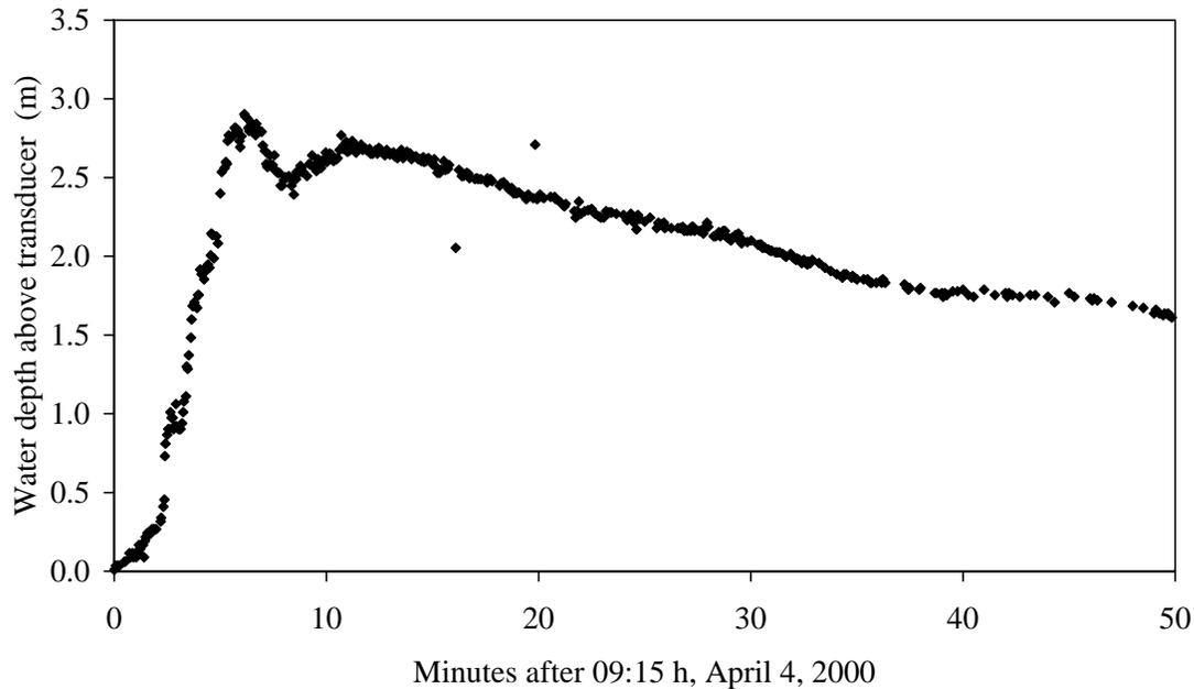
Figure 4. Stage recorded on the Restigouche River on April 4, 2000. From Beltaos and Burrell (2005a) with changes.
