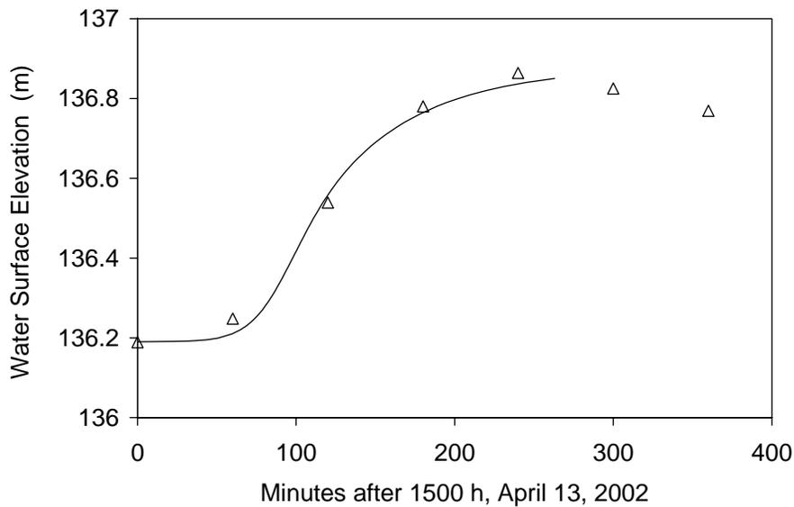
Figure 8. Comparison between calculated (line) and measured (data points) water levels during the rising portion of the Saint John River wave at Edmundston ( $C_L = 3.4$  m/s;  $C_P = 2.0$  m/s). From Beltaos and Burrell (2005b) with changes
