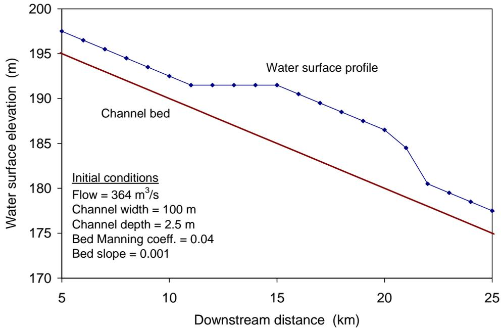
Fig. 9. Assumed initial conditions and water surface profile caused by an ice jam in an open-water reach of a hypothetical channel
