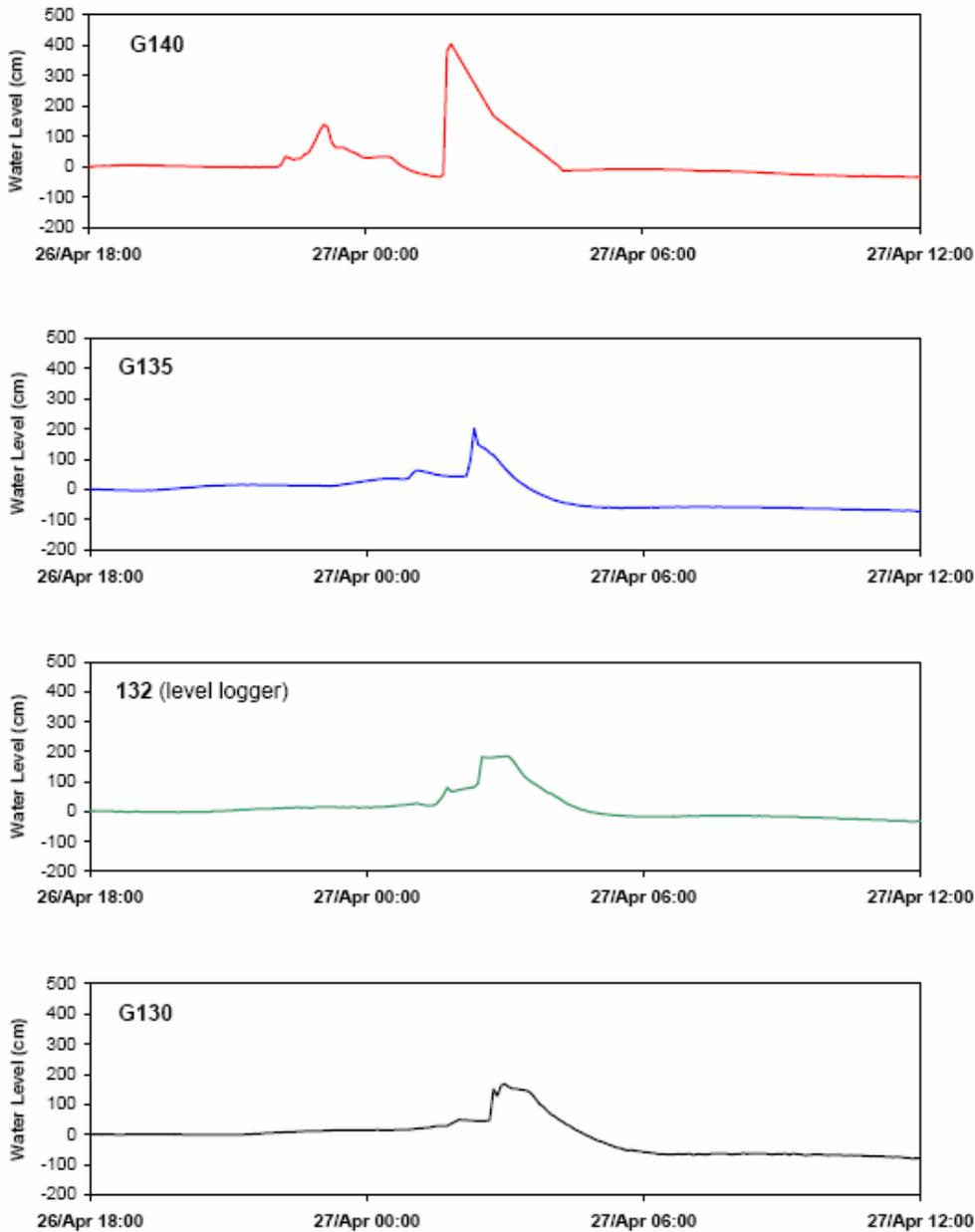
Figure 2. Waveforms obtained at consecutive monitoring stations on the Athabasca River above Fort McMurray, 2002. From Kowalczyk and Hicks (2003). Note progressive wave attenuation and dispersal.
