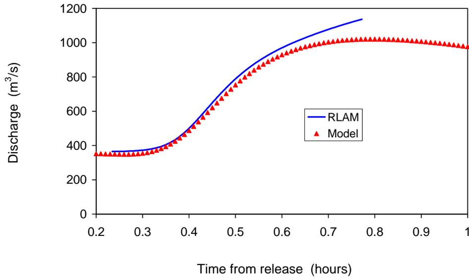
Fig. 11. Comparison between analytically-derived and model-generated flows at a site located 7 km below the toe of the jam
