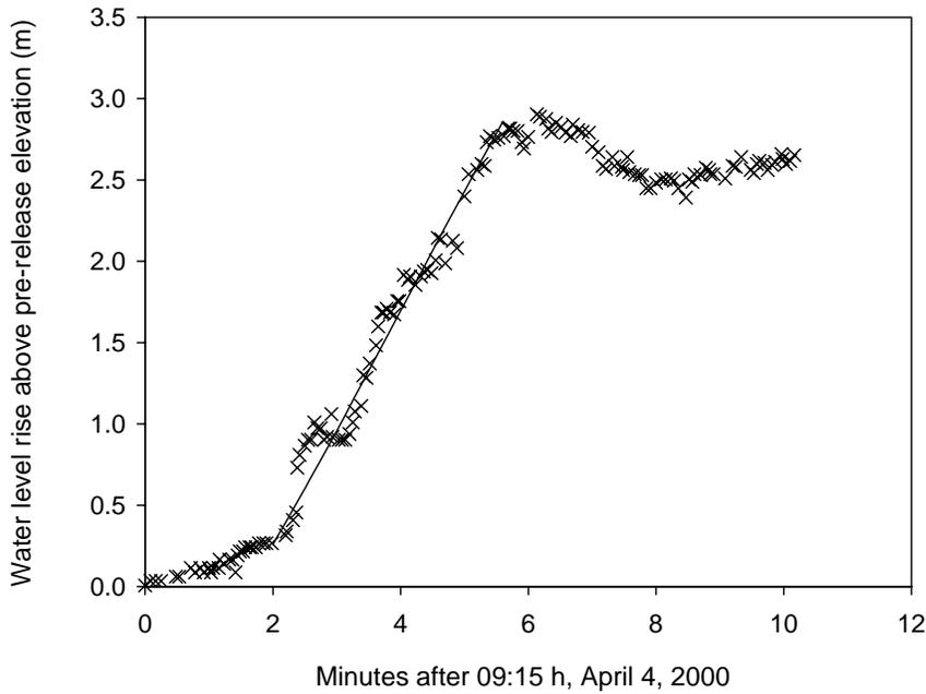
Figure 7. Comparison between calculated (line) and measured (data points) water levels during the rising portion of the Restigouche River wave at Walker's camp ( $C_L = C_P = 6.7$  m/s). From Beltaos and Burrell (2005b) with changes
