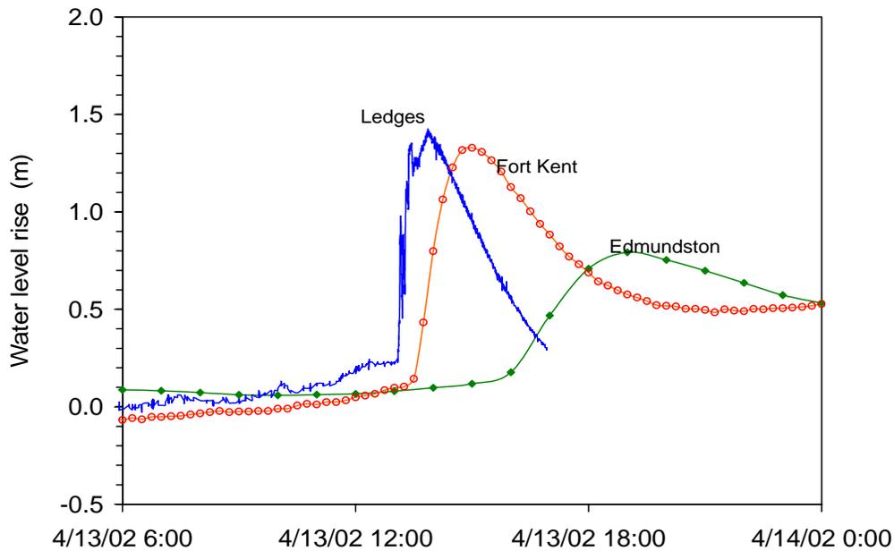
Figure 6. Saint John River surge of April 13, 2002, as registered at Ledges, Fort Kent, and Edmundston. Water level rise is above an arbitrary datum in each case. From Beltaos and Burrell (2005b) with changes.
