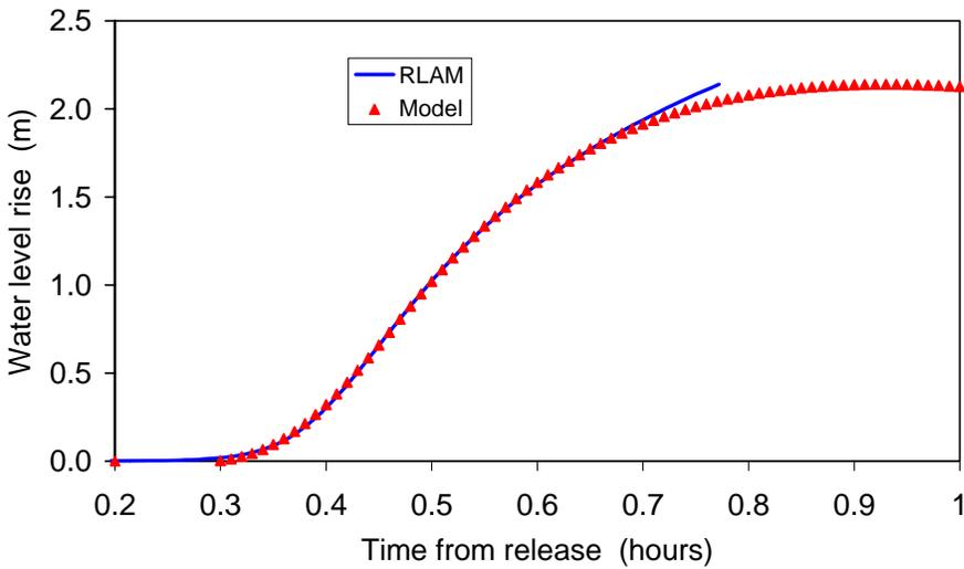
Fig. 10. Matching the rising limb of the model-generated waveform at a site located 7 km below the toe of the jam
