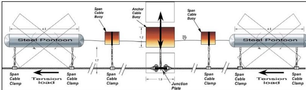
Figure 23: The Suppressed Motion of the Cut Pontoons during a Storm
