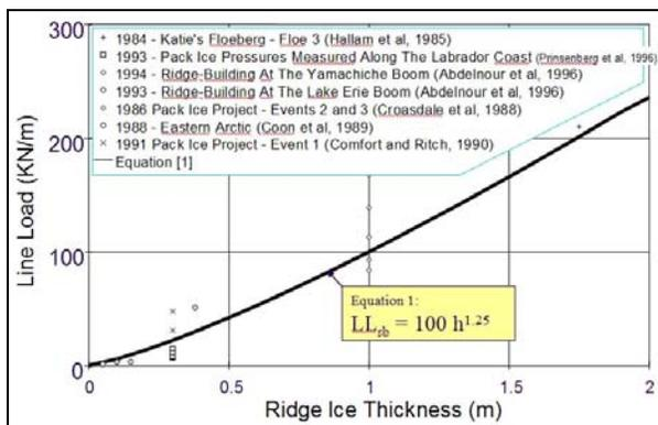
Figure 14: Pack Ice Pressure: Limiting Line Load
