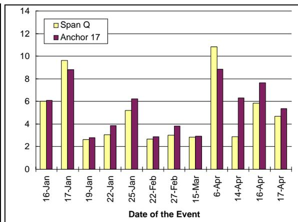
Figure 3: Line Load during 1997 Ice Run Even (Steel)
