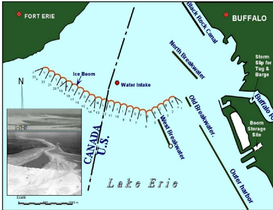
Figure 1: Location and Arrangement of Lake Erie-Niagara River Ice Boom
