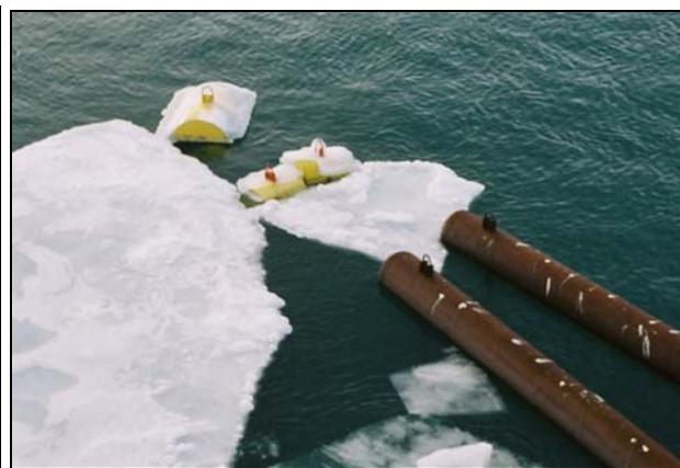
Figure 21: Consolidated Ice around the Buoys
