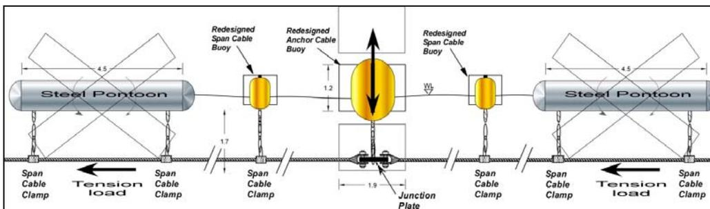
Figure 25: The Suppressed Motion of the Cut Pontoons during a Storm
