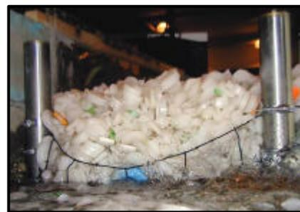
Fig. 6. Pier-net ICS near failure
