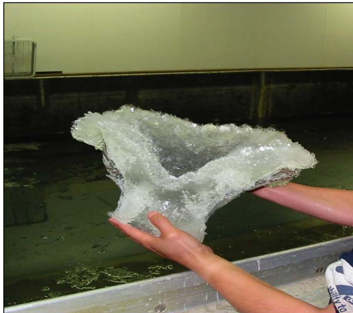
Fig. 8. Frazil ice blockage of mesh eventually caused mesh and ice to collapse into intake cone.
