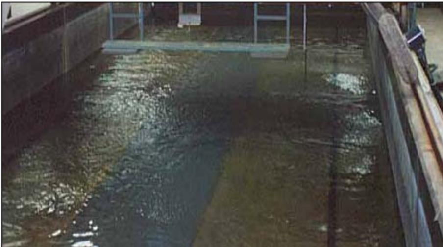
Fig. 4. Surface waves (about 25mm in height) created by fans.
