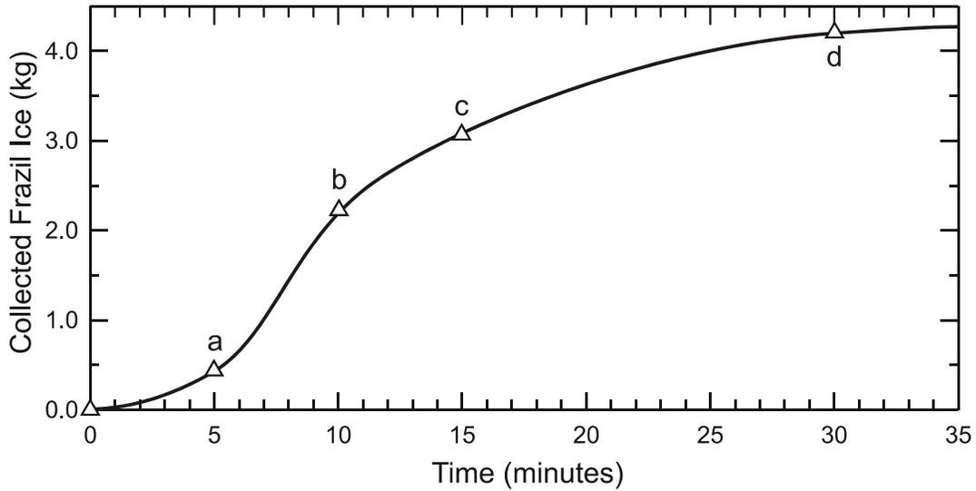
Fig. 7. Temporal rate of frazil ice accumulation on mesh.
