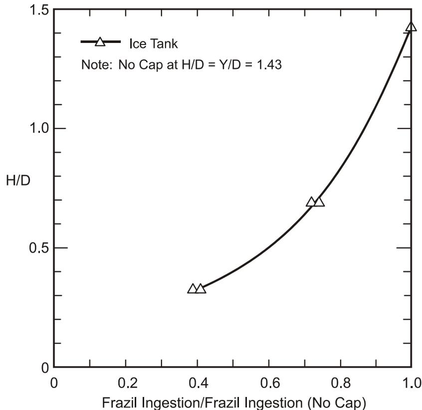
Fig. 9. Influence of intake-cap height/rim diameter (H/D) on quantity of frazil ice ingested by intake. The experiment results are taken from Table 2 for full-depth agitation.
