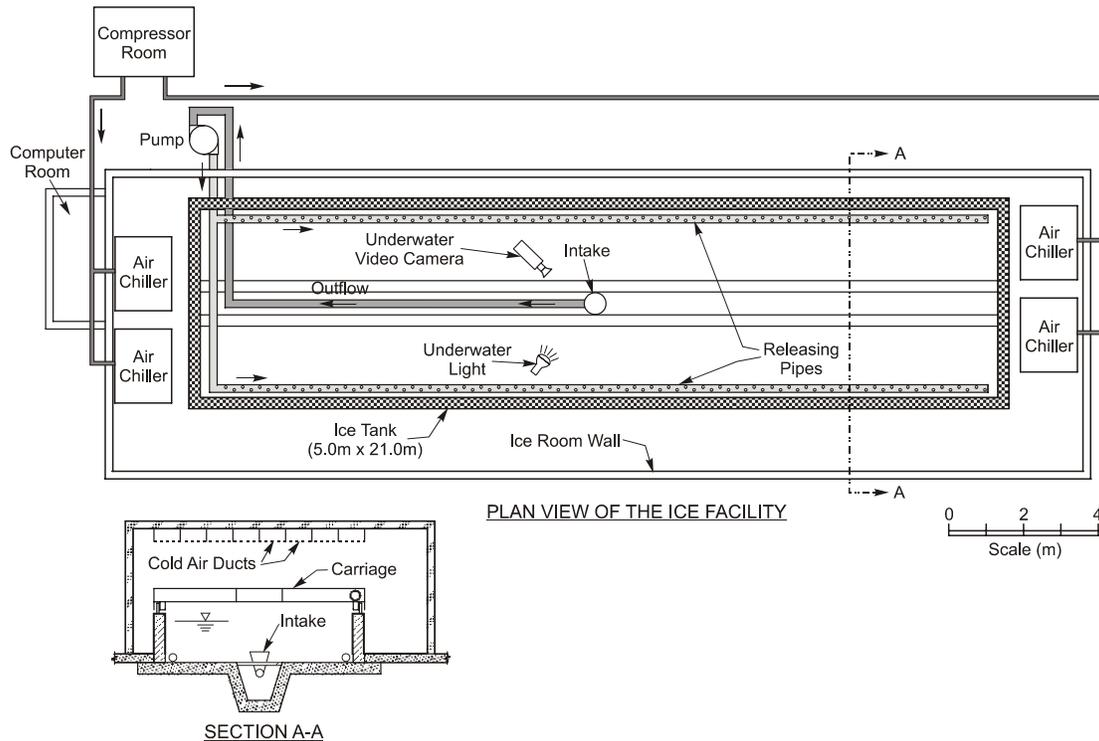
Fig. 2: Layout of ice tank and location of intake.
