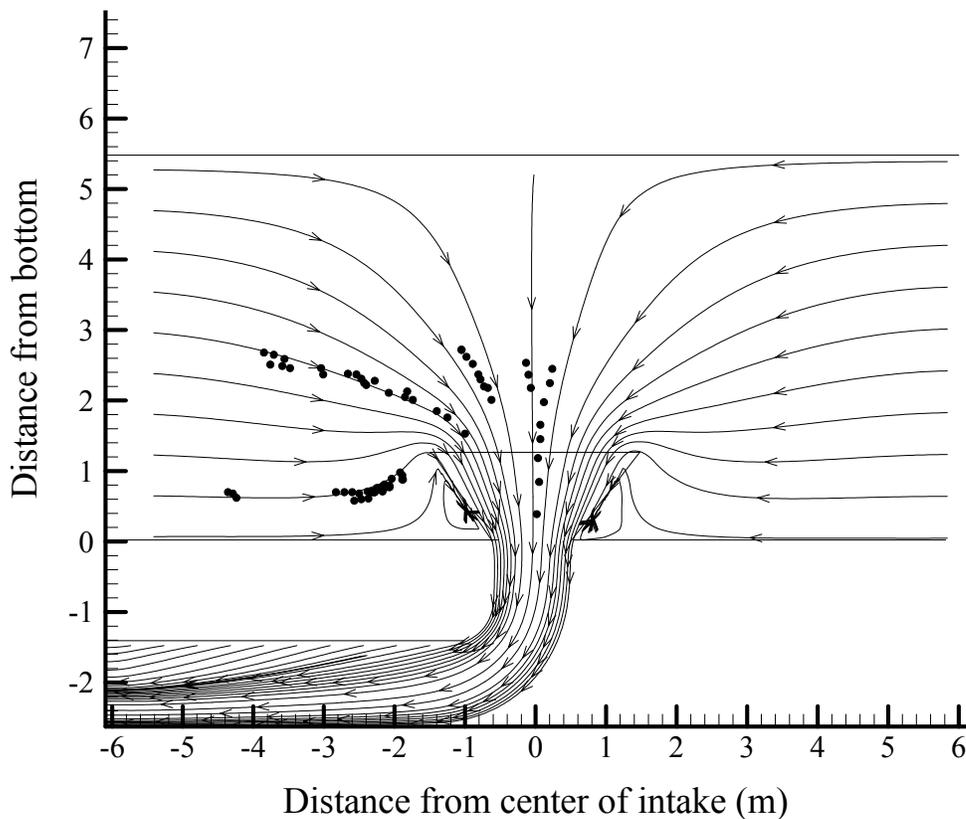
Fig. 5. Flow streamlines (numerical model) and pathlines (data from PIV measurement of dye heads) at intake.
