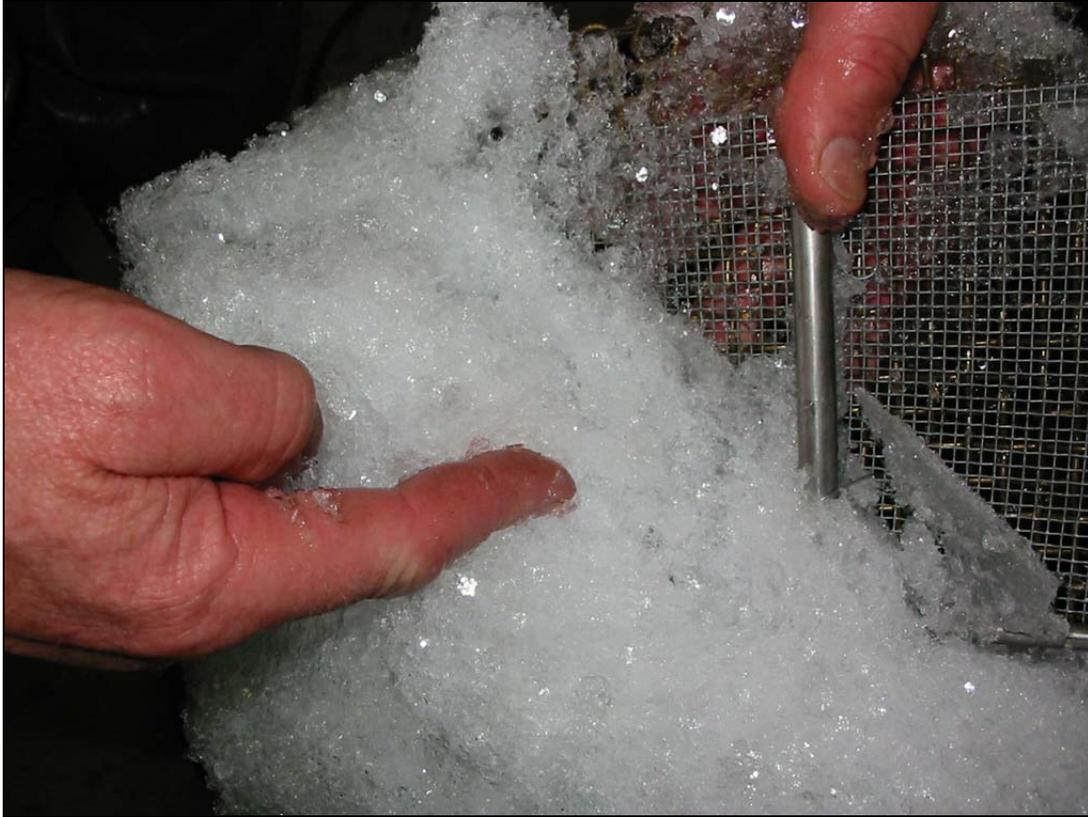
Fig. 6. Uniform-sized frazil ice crystals on collection mesh.
