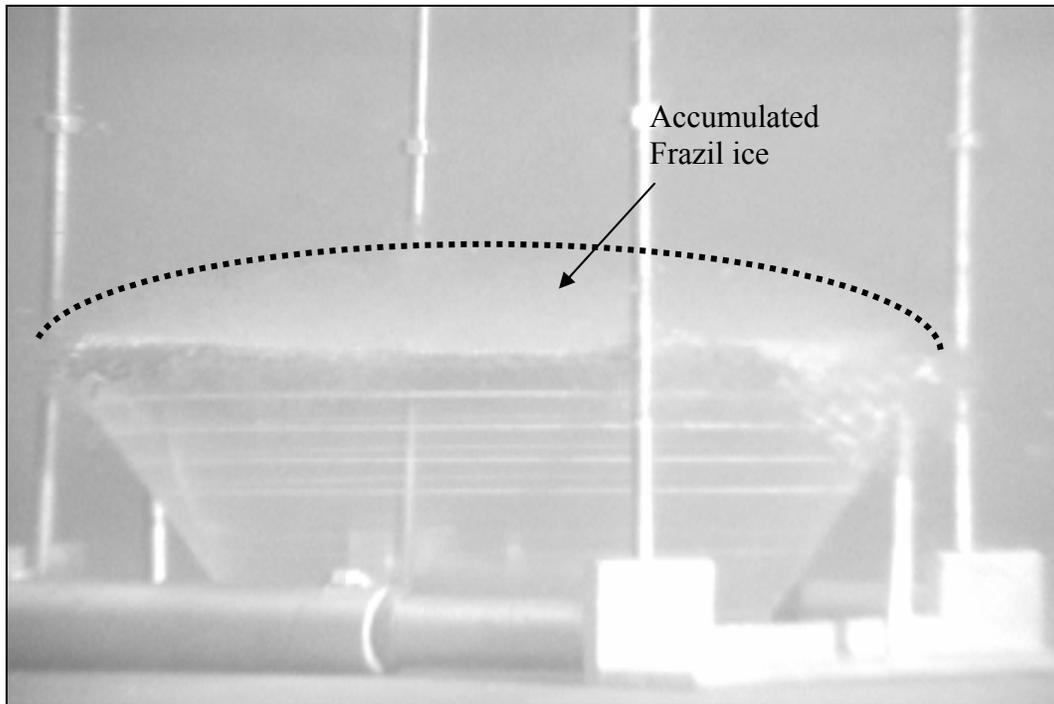
Fig. 5. Frazil ice accumulated on mesh over intake rim. The vertical posts were used to support a cap placed at variable elevation above the intake rim.
