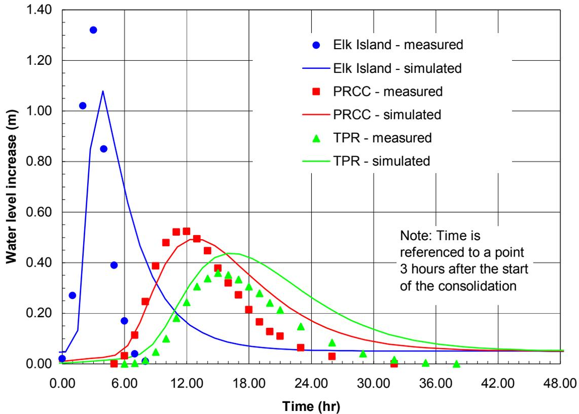
**Figure 6** Comparison of measured and simulated stage levels downstream of the consolidation
