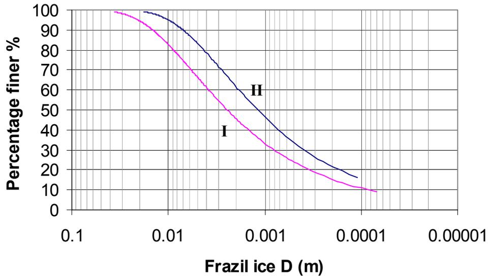
**Figure 2.** Frazil size distribution for two of Carstens' tests
