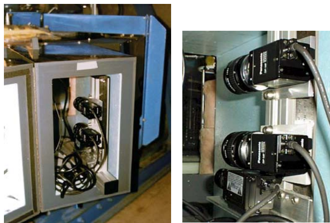
Figure 2. Array of CCD cameras used to monitor frazil ice.
