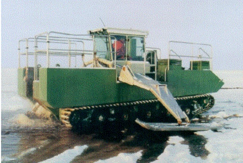
Figure 3. The ice sawing machine. (Photo by Pekka Leiviskä)
