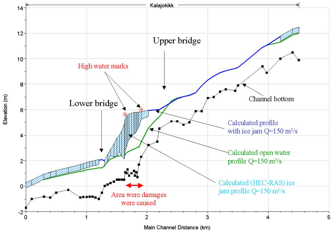
Figure 9. The longitudinal profile of the river at the main village of Kalajokki. The ice jam calculated with HEC-RAS as well as water level profiles and high water marks are presented in the figure.
