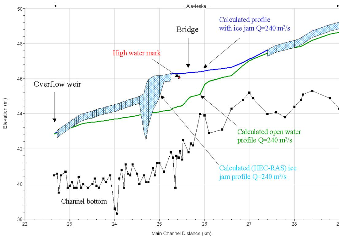
Figure 11. The longitudinal profile of the river in Alavieska. The ice jam calculated with HEC-RAS as well as water level profiles and the high water mark are presented in the figure.
