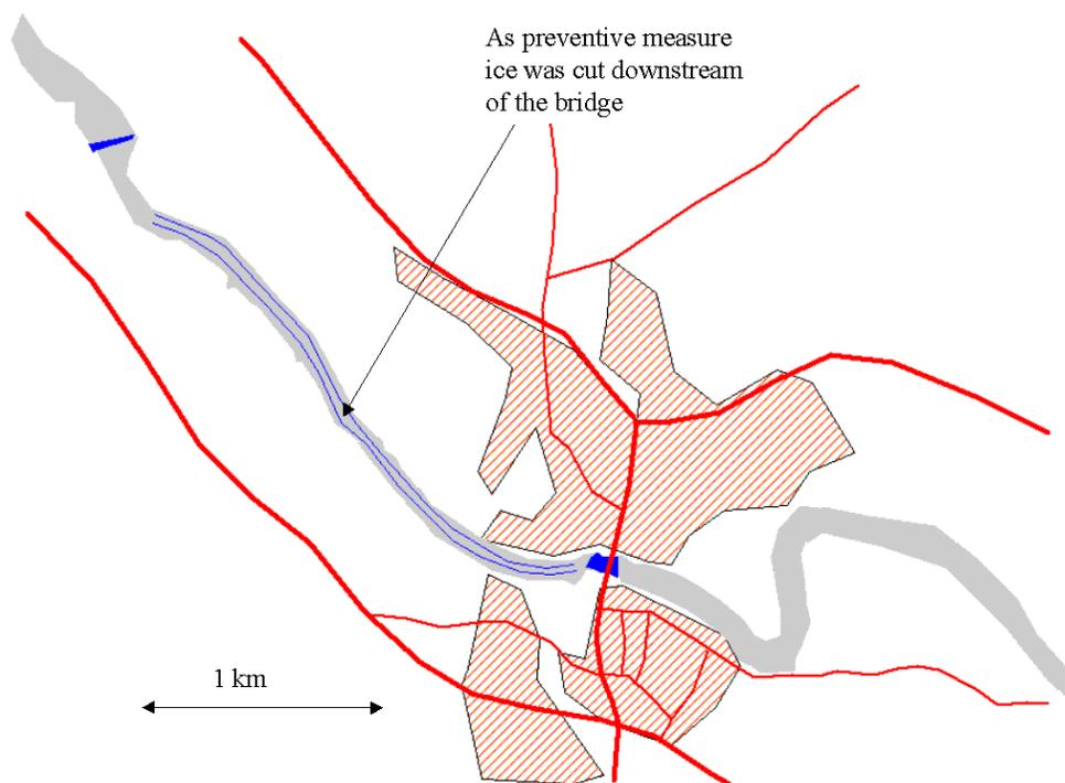
Figure 10 a. Use of ice sawing as preventive measure in Alavieska.
